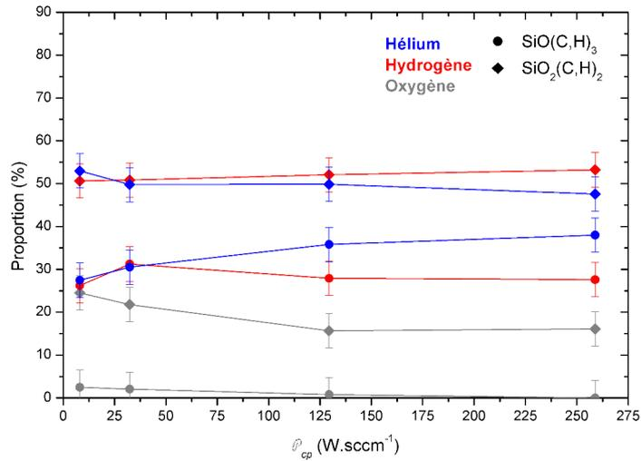
(a)  $SiO(C,H)_3$  et  $SiO_2(C,H)_2$ .
