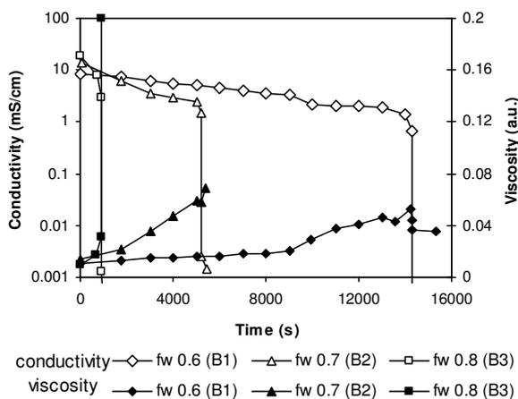
Figure 3. Conductivity and viscosity variations during the catastrophic inversion of an emulsion using the continuous stirring protocol in the  $C^+ \rightarrow A^+$  direction.  $\eta_o = 0.001$  Pa.s;  $\eta_w = 0.001$  Pa.s; (B1) fw=0.6; (B2) fw=0.7, (B3) fw=0.8.
