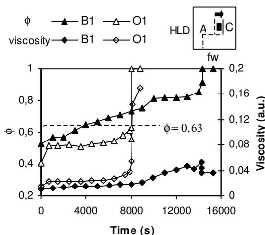
Figure 6. Variation of the dispersed phase fraction and emulsion viscosity for two oil phases. (B1)  $\eta_o = 0.001$  Pa.s;  $\eta_w = 0.001$  Pa.s; (O1)  $\eta_o = 0.02$  Pa.s;  $\eta_w = 0.001$  Pa.s.  $fw = 0.6$
