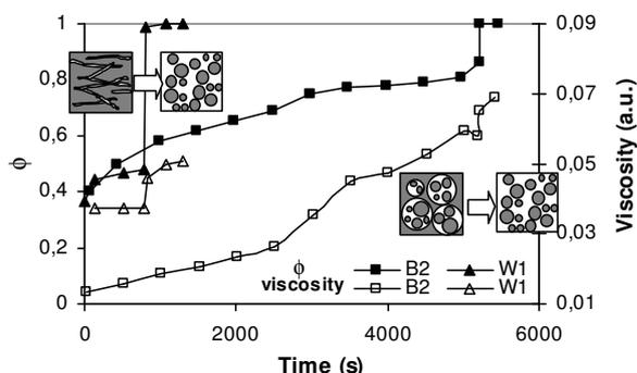
Figure 9. Viscosity follow-up and dispersed phase fraction under stirring for systems with different water viscosity. (B2)  $\eta_o = 0.001$  Pa.s,  $\eta_w = 0.001$  Pa.s; (W1)  $\eta_o = 0.02$  Pa.s,  $\eta_w = 0.001$  Pa.s.  $\phi_w = 0.7$
