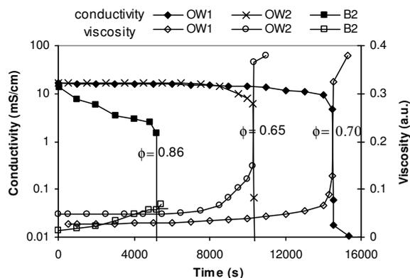
Figure 10. Conductivity and viscosity variations of an emulsion during the continuous stirring protocol for systems with the same viscosity ratio ( $R=1$ ) attained with different phase viscosities. Base case (B2)  $\eta_o = 0.001$  Pa.s,  $\eta_w = 0.001$  Pa.s; (OW1)  $\eta_o = 0.01$  Pa.s,  $\eta_w = 0.01$  Pa.s; (OW2)  $\eta_o = 0.02$  Pa.s,  $\eta_w = 0.02$  Pa.s.  $\phi_w = 0.7$ .
