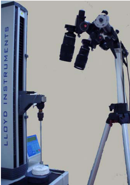
Figure 10. 3D image correlation setup
