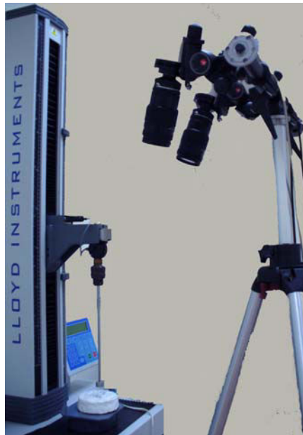
Figure 10. 3D image correlation setup
