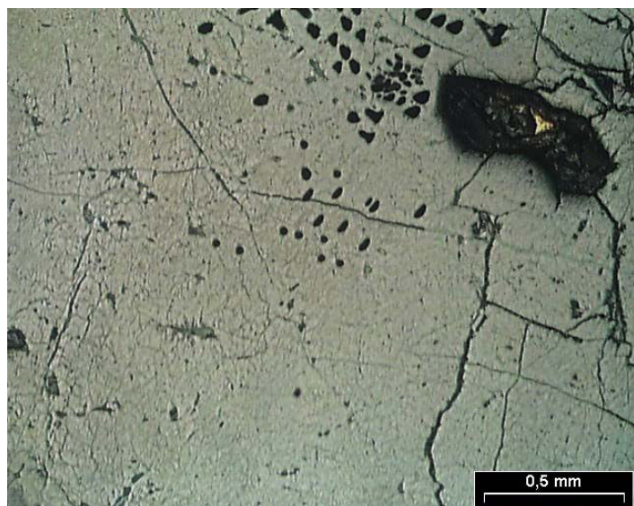
Figure 2. Optical image in reflected light microscopy of a large surface of a uraninite from the Mistamisk sample. At the top, the black spots correspond to the craters produced during ion microprobe analyses.
