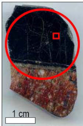
Figure 1 Localization of the polished section cut in the sample (red circle). Red square: TEM sampling area.
