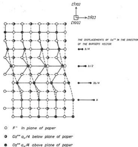
**Figure II.14:** A screw dislocation on  $\{100\}\langle 011\rangle$  [29].
