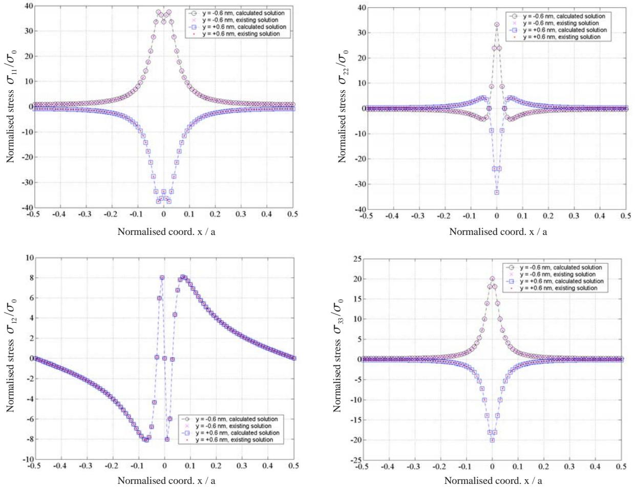
**Figure X.7:** Comparison of calculated stress components for an edge dislocation pile-up in a unit cell (defined in Fig. X.2) obtained by means of the new tool (Eq. X.15) with the simplified solution provided in the open literature [22].
