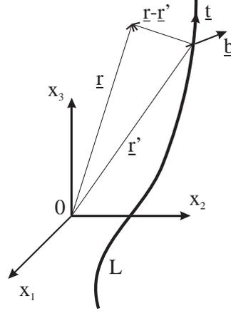
Figure IX.6: Parametrisation of a single dislocation line.
