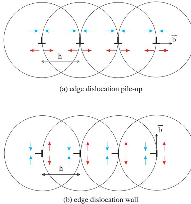
**Figure X.15:** Simplified representation of tensile and compressive fields in the edge dislocation pile-up and wall configurations.
