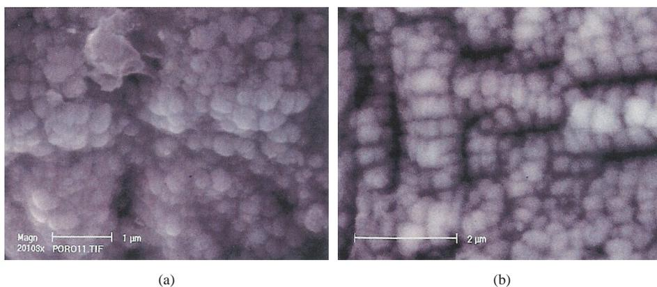
**Figure IV.9:** SEM micrographs showing round sub-grains: (a) disordered round grains at the surface of a pore, and (b) grain surface sub-division on rolls, which are sub-divided on ordered round grains [63].
