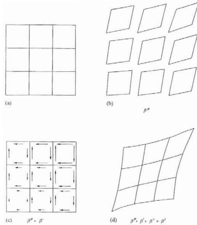
**Figure IX.4:** Incompatibility of elastic and plastic strains [51].
