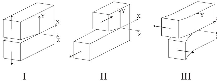
Figure V.1: The three fundamental types of crack opening.
