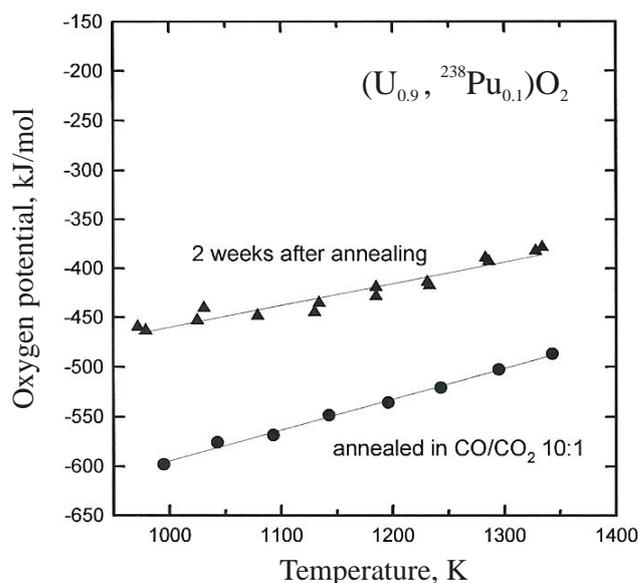
**Figure XIII.4:** Oxygen potential of the  $(U_{0.9}, Pu_{0.1})O_2$  sample as a function of temperature, measured immediately after annealing and 2 weeks after [114].
