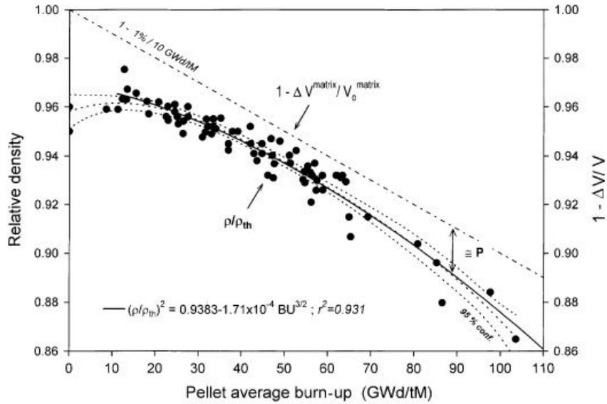
**Figure IV.7:** Measured relative immersion density as a function of the average pellet burn-up [127].  $\rho$  is the bulk fuel density,  $\rho_{th}$  the theoretical density of  $\text{UO}_2$  ( $10.96 \text{ g}\cdot\text{cm}^{-3}$ ), and  $\Delta V^{matrix}/V_0^{matrix}$  represents the fuel matrix swelling (split into the contributions of solid and gaseous fission products).
