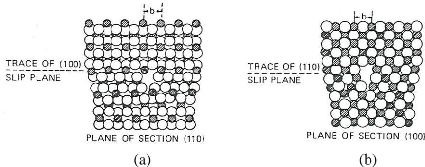
**Figure II.13:** Atomic configurations around edge dislocations in  $\text{UO}_2$  on (a) the primary slip system  $\{100\}\langle 110\rangle$ , (b) the secondary slip system  $\{110\}\langle 110\rangle$  [116]. The U atoms are in black and the O ones in white.
