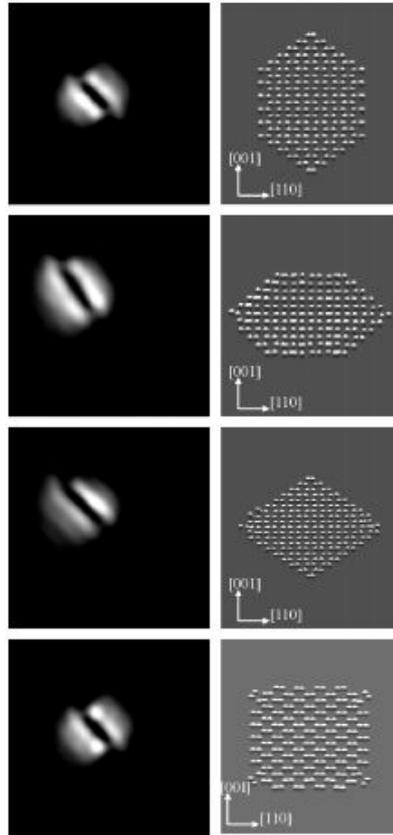
**Figure XIII.6:** Simulated images (left) of  $\langle 100 \rangle \{110\}$  loops with different sizes and shapes (right) in  $\alpha$ -Fe. The atomic configurations on the right are viewed from a  $[1\bar{1}0]$  direction [68].
