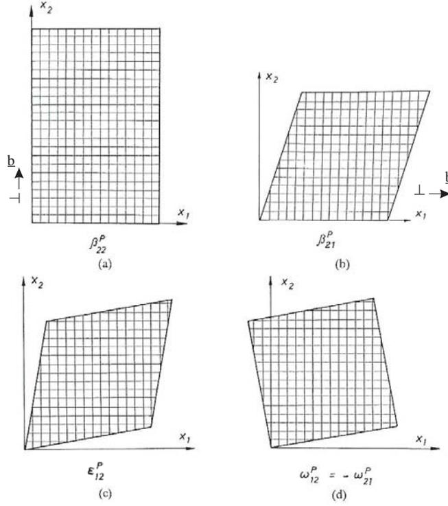
**Figure IX.3:** Examples of macroscopically homogeneous plastic distortions of the crystal in Fig. IX.1 [51].
