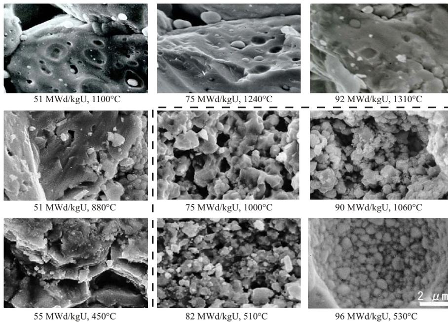
**Figure IV.11:** SEM observations on the fracture surfaces of specimens irradiated at different burn-ups and temperatures. All pictures have same magnification. The dashed line shows the threshold for the HBS formation [118].
