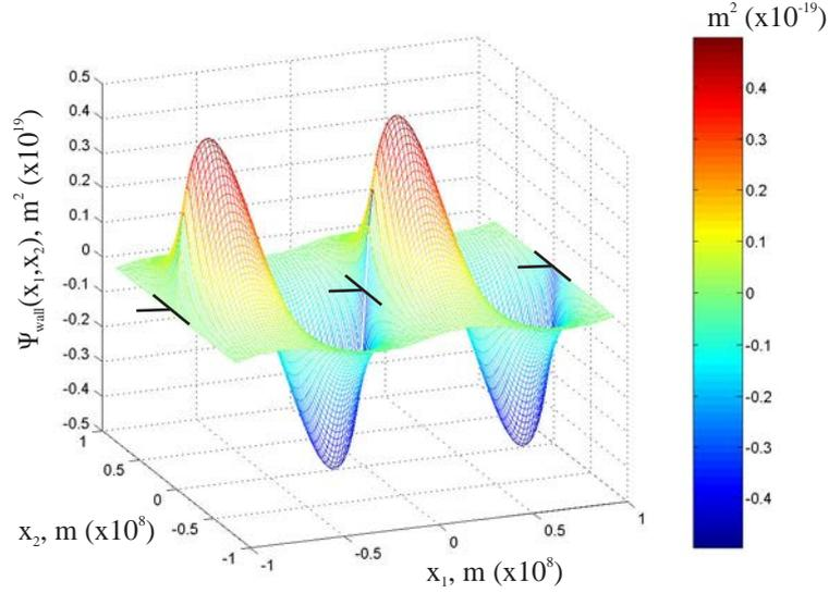
**Figure X.6:**  $\psi_{wall}(x_1, x_2)$  for an edge dislocation wall.
