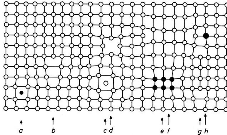
**Figure II.3:** Various crystal lattice defects: (a) interstitial impurity atom, (b) edge dislocation, (c) self-interstitial atom, (d) vacancy, (e) precipitate of impurity atoms, (f) vacancy-type dislocation loop, (g) interstitial-type dislocation loop, (h) substitutional impurity atom
