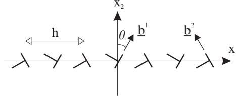
Figure X.12: Symmetrical tilt-boundary.
