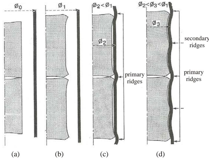
**Figure III.6:** Evolution of the gap between the cladding and the fuel pellet during irradiation. (a) start of irradiation, (b) first cycle and start of second irradiation cycle, (c) second half of second cycle: first cladding-pellet contact and appearance of primary ridges, (d) in case of power ramp: appearance of secondary ridges [5].
