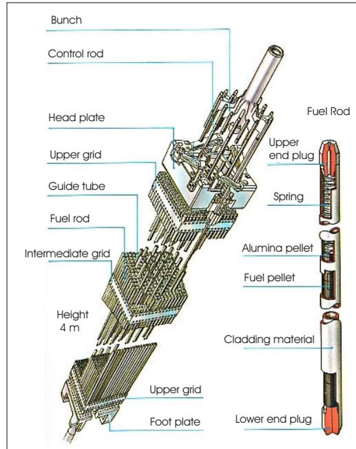
**Figure I.2:** Fuel rod assembly of a PWR.
