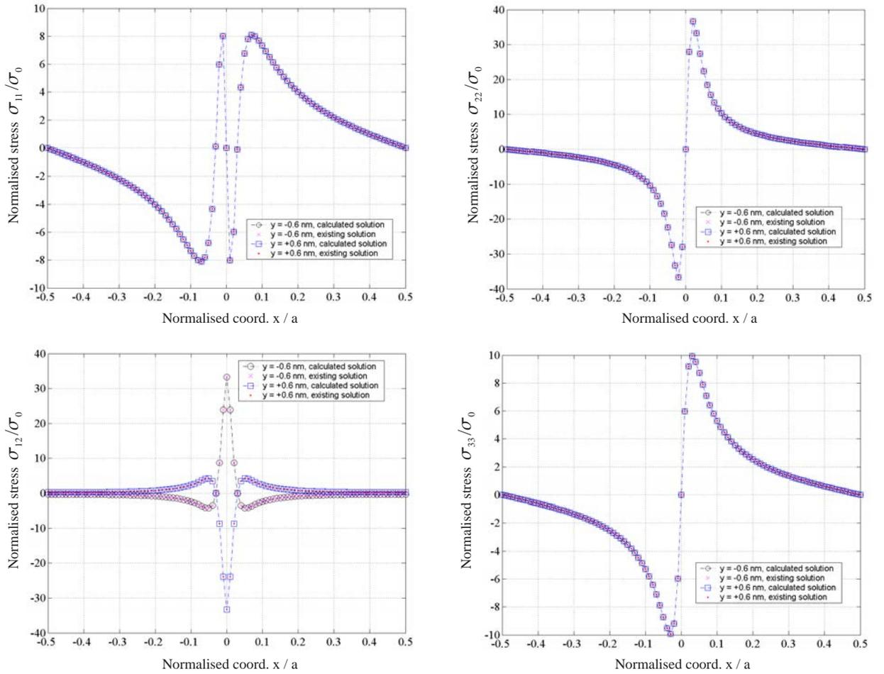
**Figure X.8:** Comparison of calculated stress components for an edge dislocation wall in a unit cell (defined in Fig. X.4) obtained by means of the new tool (Eq. X.28) with the simplified solution provided in the open litterature [22].
