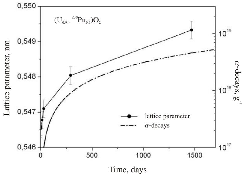
**Figure XIII.2:** Lattice parameter changes as a function of time [24]. The  $\alpha$ -decay evolution with time for  $^{238}\text{Pu}$  is also shown.
