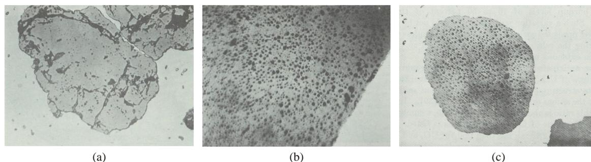
**Figure IV.2:** Metallographs of (a) unirradiated  $\text{UO}_2$  particle of 95%TD in stainless-steel matrix, as-etched, (b) irradiated to 25 at%, as-polished, (c) irradiated to 30 at%, as-polished. All pictures are  $\times 500$ , reduction factor 1/2 [8].
