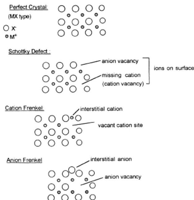
**Figure II.4:** Point defects in an MX-type ionic crystal.
