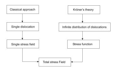
Figure X.1: Stress calculation methods.
