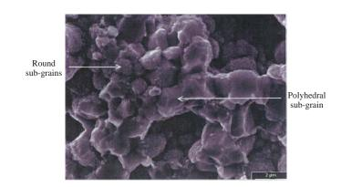
Figure IV.8: SEM micrograph showing the two different types of grains observed in the HBS. The HBS has been observed in the  $PuO_2$  agglomerates of a MOX fuel [62].
