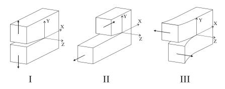
Figure V.1: The three fundamental types of crack opening.
