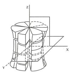
Figure III.5: Fuel pellet with a "hourglassing" shape due to the effect of thermal stresses [5].
