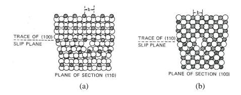
Figure II.13: Atomic configurations around edge dislocations in UO<sub>2</sub> on (a) the primary slip system  $\{100\} < 110 >$ , (b) the secondary slip system  $\{110\} < 110 >$  [116]. The U atoms are in black and the O ones in white.
