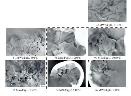
Figure IV.12: TEM micrographs of specimens irradiated at different burn-ups and temperatures. All pictures have same magnification [119].
