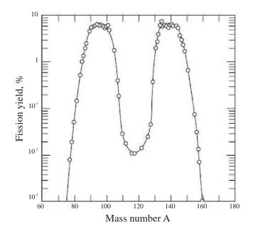
Figure II.2: Fission product distribution of thermal neutron fission of <sup>235</sup>U.
