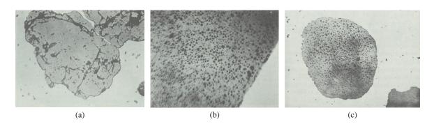
Figure IV.2: Metallographs of (a) unirradiated UO<sub>2</sub> particle of 95%TD in stainless-steel matrix, as-etched, (b) irradiated to 25 at%, as-polished, (c) irradiated to 30 at%, as-polished. All pictures are ×500, reduction factor 1/2 [8].
