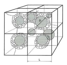
Figure VI.2: Cellular representation of the HBS as proposed by Spino et al. [129].
