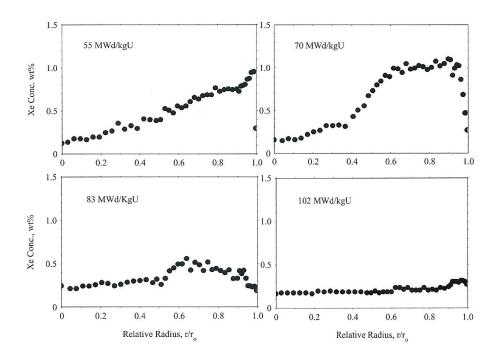
Figure IV.3: EPMA concentration profiles for the radial distribution of Xe retained in the  $UO_2$  grains of 4 PWR fuels [20].
