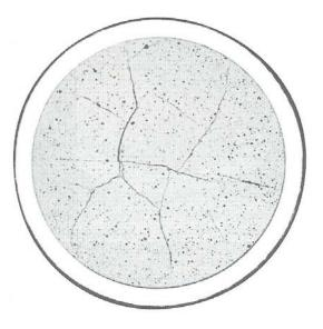
Figure III.4: Macrography of a PWR fuel pellet cracked by the thermal gradient [5].
