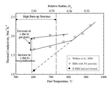
Figure V.5: Thermal conductivity of the high burn-up fuel at  $217^{\circ}$ C as a function of the local radial temperature during the last irradiation cycle [144].
