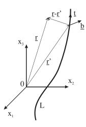
Figure IX.6: Parametrisation of a single dislocation line.
