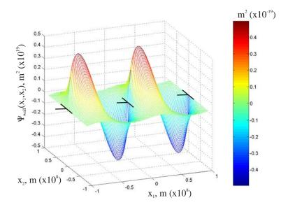
**Figure X.6**:  $\psi_{wall}(x_1, x_2)$  for an edge dislocation wall.
