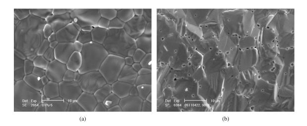
**Figure XIII.1**: SEM micrographs of the fabricated  $(U_{0.9}, Pu_{0.1})O_2$  sample showing (a) grain-boundaries thermally etched, and (b) a transgranular fracture.
