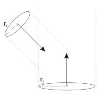
Figure XIV.2: Coalescence of two loops of different radius, diffusing along one of the (110) planes. The resulting loop is assumed to be cylindrical.
