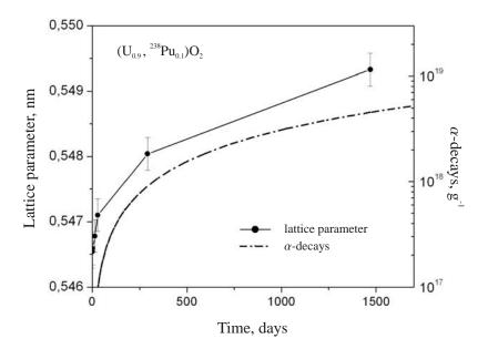
Figure XIII.2: Lattice parameter changes as a function of time [24]. The  $\alpha$ -decay evolution with time for <sup>238</sup>Pu is also shown.
