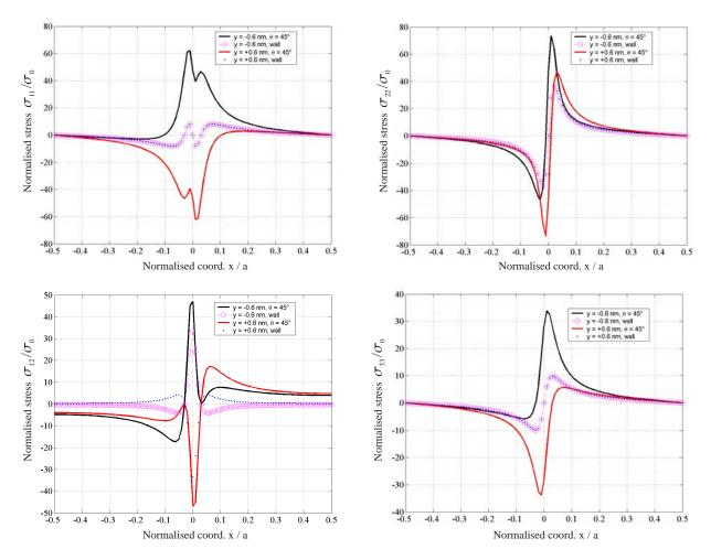
Figure X.13: Calculated stress components for a symmetrical tilt-boundary. The components are plotted for the dislocation line situated in  $x_1=0$ . The stress components of the edge dislocation wall are also shown.
