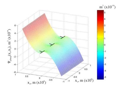
**Figure X.5**:  $\psi_{pileup}(x_1, x_2)$  for an edge dislocation pile-up.
