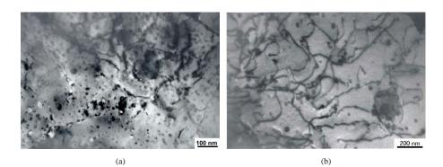
Figure IV.14: TEM micrographs of non-restructured UO<sub>2</sub> of (a) 55 MWd/kgU,  $450^{\circ}$ C and (b) 92 MWd/kgU,  $1310^{\circ}$ C [119].
