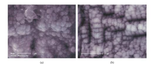
Figure IV.9: SEM micrographs showing round sub-grains: (a) disordered round grains at the surface of a pore, and (b) grain surface sub-division on rolls, which are sub-divided on ordered round grains [63].
