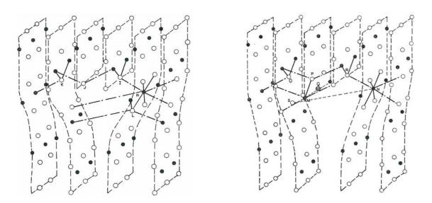
Figure II.11: The negatively charged configuration [29]. Figure II.12: The uncharged configuration [29].
