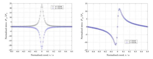
Figure X.11: Calculated solutions of stress components for a screw dislocation pile-up as defined by Fig. X.10.
