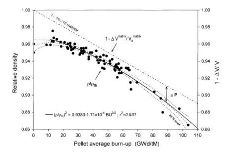
**Figure IV.7**: Measured relative immersion density as a function of the average pellet burn-up [127].  $\rho$  is the bulk fuel density,  $\rho_{th}$  the theoretical density of UO<sub>2</sub> (10.96 g.cm<sup>-3</sup>), and  $\Delta V^{matrix}/V_0^{matrix}$  represents the fuel matrix swelling (split into the contributions of solid and gaseous fission products).
