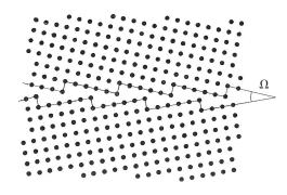
Figure X.18: Lattice representation of a low-angle  $\theta$  grain-boundary.
