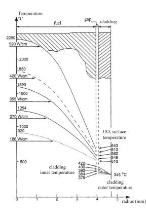
Figure III.3: Temperature distribution in a PWR fuel pellet as function of linear power [55].
