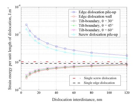
Figure X.14: Elastic energy in a unit cell, per unit length of dislocation. The length of the unit cell along  $x_2$  has been chosen to be constant for all configurations and equal to 320 nm in order to take into account possible long range stresses.
