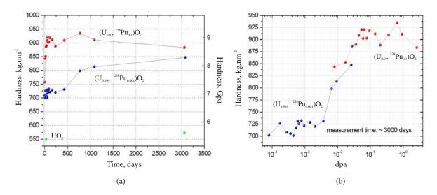
Figure XIII.3: Vickers hardness as a function of time (a), and dpa (b), for the  $(U_{0.9}, Pu_{0.1})O_2$  and  $(U_{0.999}, Pu_{0.001})O_2$  materials [24].
