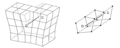
Figure II.7: Perspective view of a screw dislocation in a cubic lattice.
