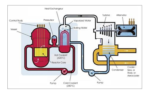
Figure I.1: Main elements of a PWR.
