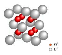
Figure II.5: UO<sub>2</sub> unit cell.
