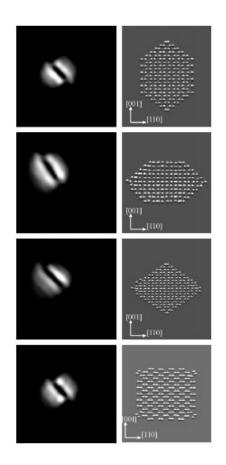
**Figure XIII.6**: Simulated images (left) of  $\langle 100 \rangle \{110\}$  loops with different sizes and shapes (right) in  $\alpha$ -Fe. The atomic configurations on the right are viewed from a [110] direction [68].
