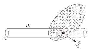
Figure XIV.1: Re-solution of interstitials from a loop back into the matrix.
