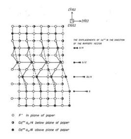
Figure II.14: A screw dislocation on {100}<011> [29].
