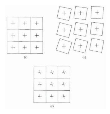
Figure IX.5: Strain-free lattice curvature [51].
