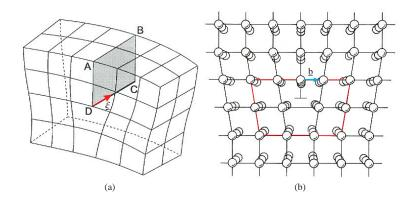
Figure II.6: Perspective view of an edge dislocation in a cubic lattice.
