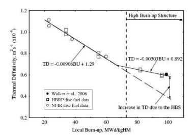
Figure V.4: Influence of the presence of the HBS on the thermal diffusivity of the high burn-up fuel. The vertical broken line marks the burn-up at which the HBRP disc fuel had fully transformed to the HBS [144].
