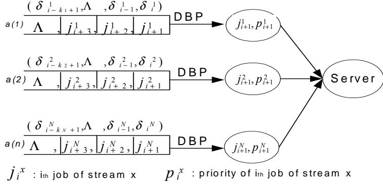
**Fig. 4: DBP for priority assignment of head-of-queue's tasks**
