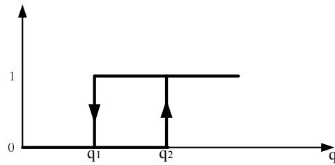
**Fig. 46 : “Double Thresholds Control” function of the switch**
