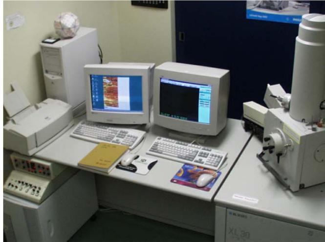
Figure III-10: Microscope Electronique à Balayage Philip XL30 SFEG.
