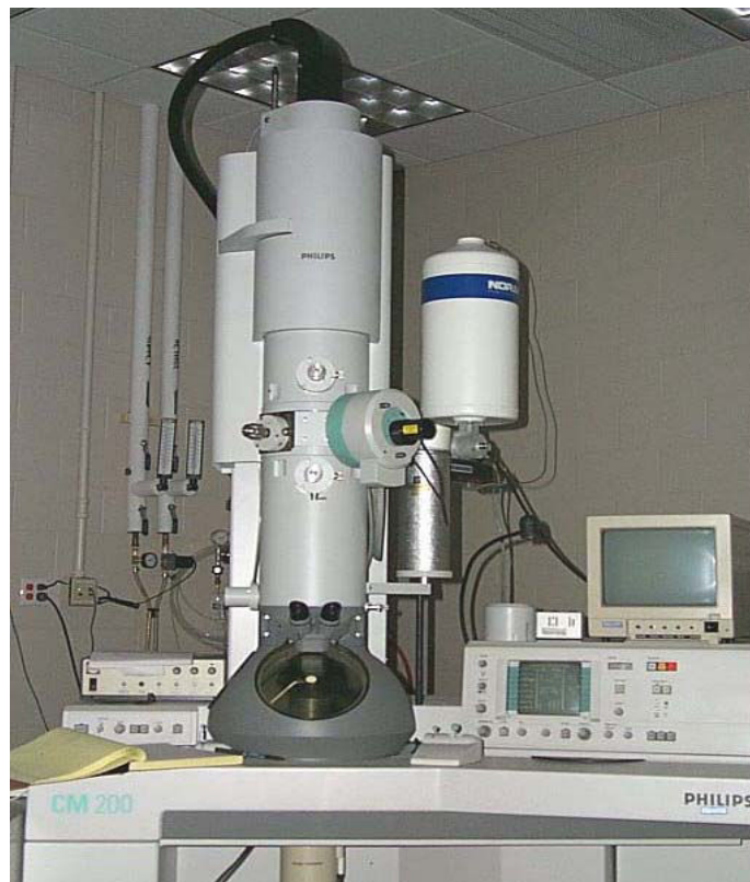
Figure III-11: Microscope Electronique à Transmission TEM Philips CM200.
