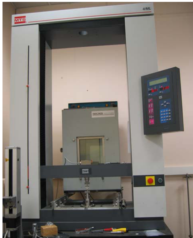
Figure III-14 : Machine de traction MTS-4/ML.
