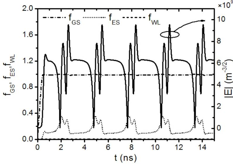
Figure 4.18: Temporal changes of the occupation probabilities of the respective energy levels when the slave laser exhibits double-pulse self-pulsations ( $\Delta = 9.4$  GHz,  $S_m = 6 \times 10^{-4}$  J/m<sup>3</sup>)
