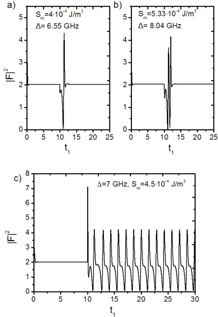
Figure 4.11: Example of triggered a) single-pulse excitability ( $\Delta = 6.55 \text{ GHz}$ ,  $S_m = 4 \times 10^{-4} \text{ J/m}^3$ ) b) double-pulse excitability ( $\Delta = 8.04 \text{ GHz}$ ,  $S_m = 5.33 \times 10^{-4} \text{ J/m}^3$ ). c) Bistability between the attractor corresponding to the locked state and the attracting limit cycle associated with the self-pulsations inside the homoclinic tooth.  $S_m = 4.5 \times 10^{-4} \text{ J/m}^3$ ,  $\Delta = 7.0 \text{ GHz}$ .
