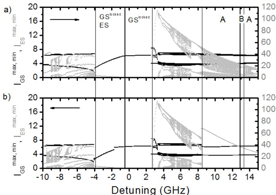
Figure 5.3: 1-parameter bifurcation diagram for  $J = 17$ ,  $S_m = 1.5 \times 10^{-4} \text{ J/m}^3$  when sweeping the detuning either from a) negative to positive or b) from positive to negative values.
