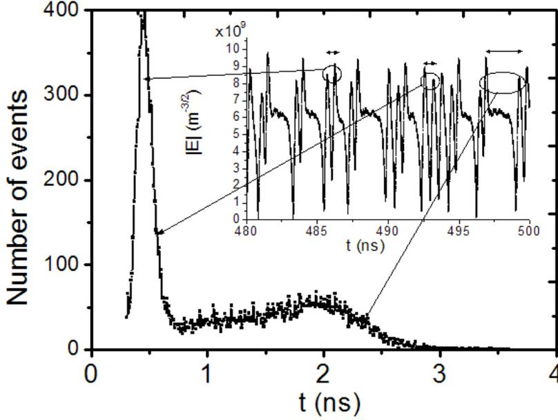
Figure 4.20: Statistics of the interpose time for the double pulse self-pulsations. ( $\Delta = 9.6$  GHz,  $S_m = \times 10^{-4}$  J/m<sup>3</sup>)
