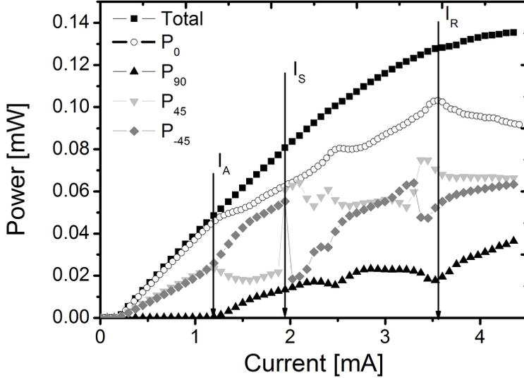
Figure 3.1: Polarization resolved power-current characteristics of the investigated QD VCSEL.
