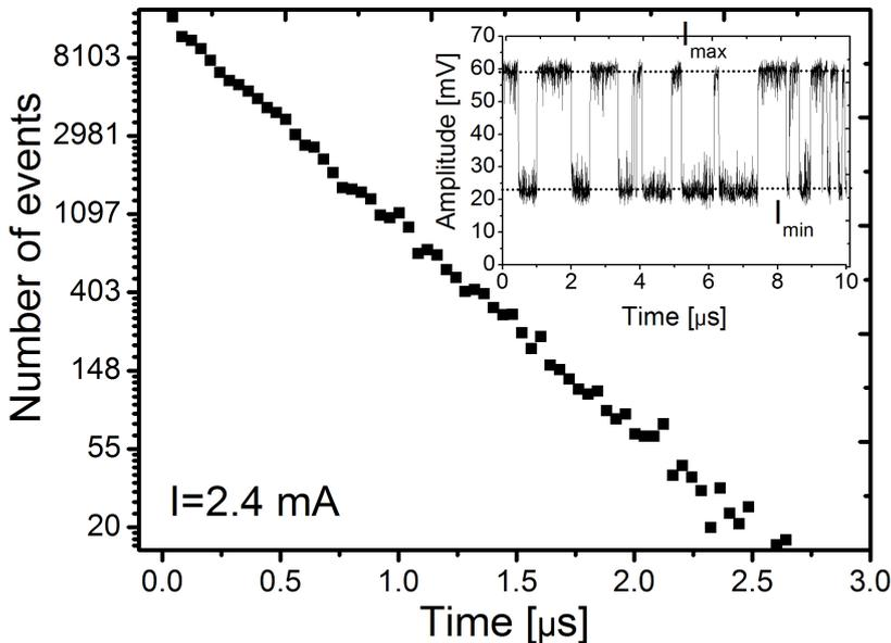
Figure 2.16: Semi-logarithmic plot for dwell time statistics at the current of 2.4 mA. The inset shows an example of time trace of the output power projected on the transmission axis of the polarizer of 45 deg.
