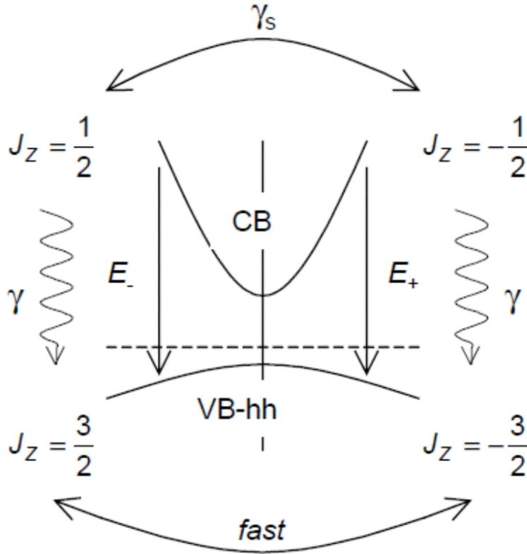
Figure 2.3: Four level system of SFM model. CB - conduction band and VB - hh - heavy hole band are split into different spin sublevels. The reservoirs of spin-up and spin-down carriers are coupled through the spin-flip processes which always tend to equalize their populations with the characteristic spin-flip rate  $\gamma_s$ . Taken from [118].
