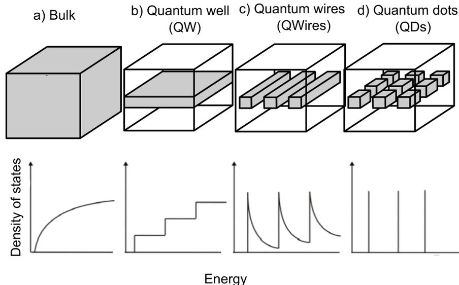
Figure 1.2: Schematic representation of the nanostructures and the corresponding density of states. a) Bulk, b) quantum well (QW), c) quantum wire (QWire), d) quantum dot (QD).
