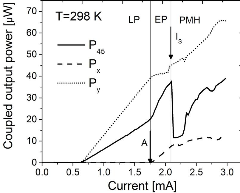
Figure 2.13: Polarization resolved power-current characteristics of SML QD VCSEL showing polarization instabilities. Polarization angle is denoted as a subscript, e.g.  $P_{45}$  means 45 deg with respect to the  $y$  axis.
