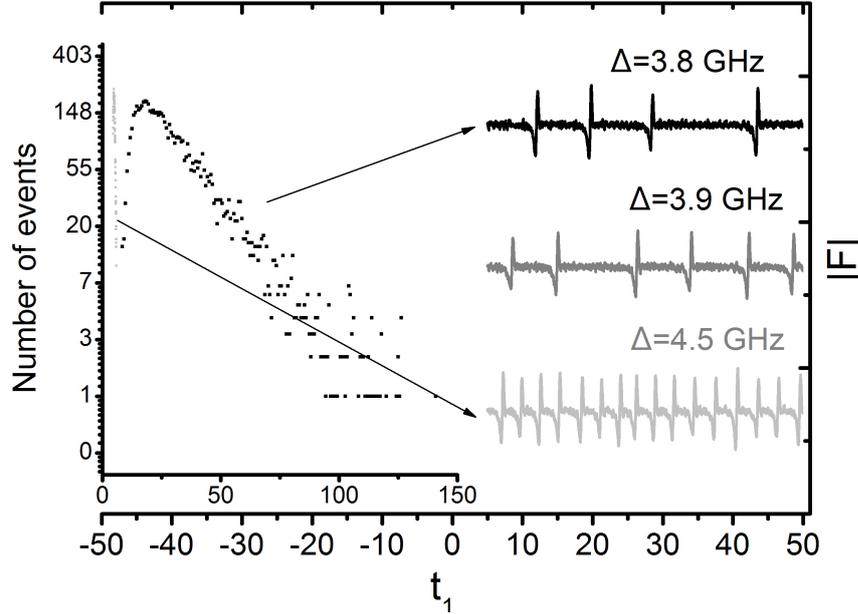
Figure 4.19: Time traces for different values of the detuning in the presence of spontaneous emission noise,  $S_m = 10^{-4}$  J/m<sup>3</sup>. The inset: semi-logarithmic plot for the distribution of the interpose time for the detuning of 3.8 GHz (black distribution) and 4.5 GHz (gray distribution).
