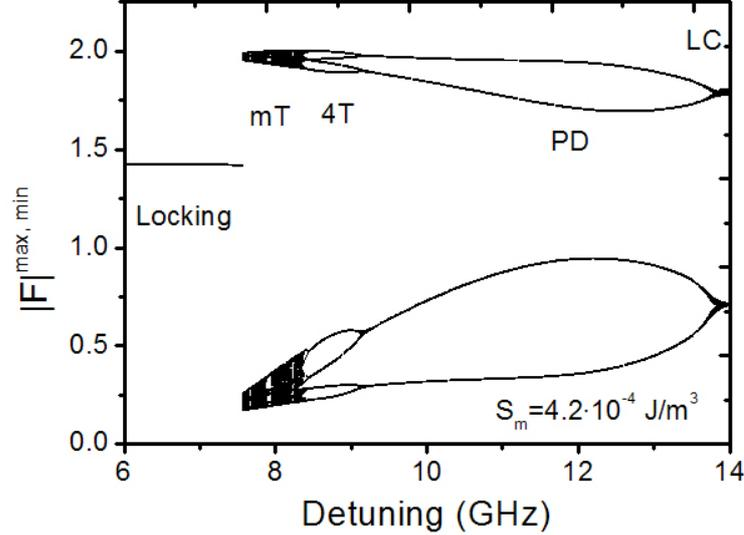
Figure 4.15: 1-parameter bifurcation diagram for  $S_m = 4.2 \times 10^{-4} \text{ J/m}^3$ .
