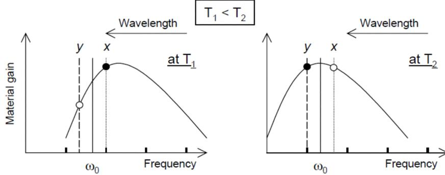
Figure 2.4: Schematic representation of type-I polarization switching due to current heating induced redshift of the cavity resonance  $\omega_0$  with respect to the peak gain frequency.  $x$  and  $y$  correspond to the linearly polarized, orthogonal modes. Taken from [118].
