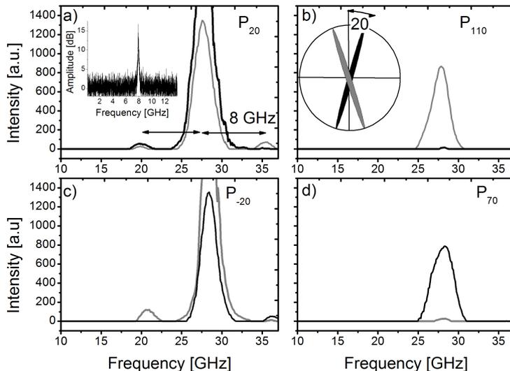
Figure 3.2: Polarization resolved optical spectra at  $I = 1.85$  mA for different orientations of the polarizer ( $P$ ). The inset in panel a) shows RF spectrum captured at  $P_{45}$ . Polarization angle is denoted as a subscript, e.g.  $P_{20}$  means 20 deg with respect to the  $y$  axis
