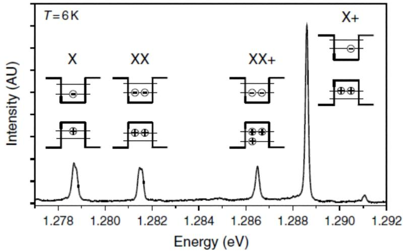
Figure 2.7: Cathodoluminescence spectra of a single-InAs quantum dot in a GaAs matrix. The emission lines correspond to different excitonic complexes, i.e.  $X$  excitons,  $XX$  biexcitons,  $XX^+$  positively charged biexcitons,  $X^+$ , positively charged excitons (trion). Taken from [130].
