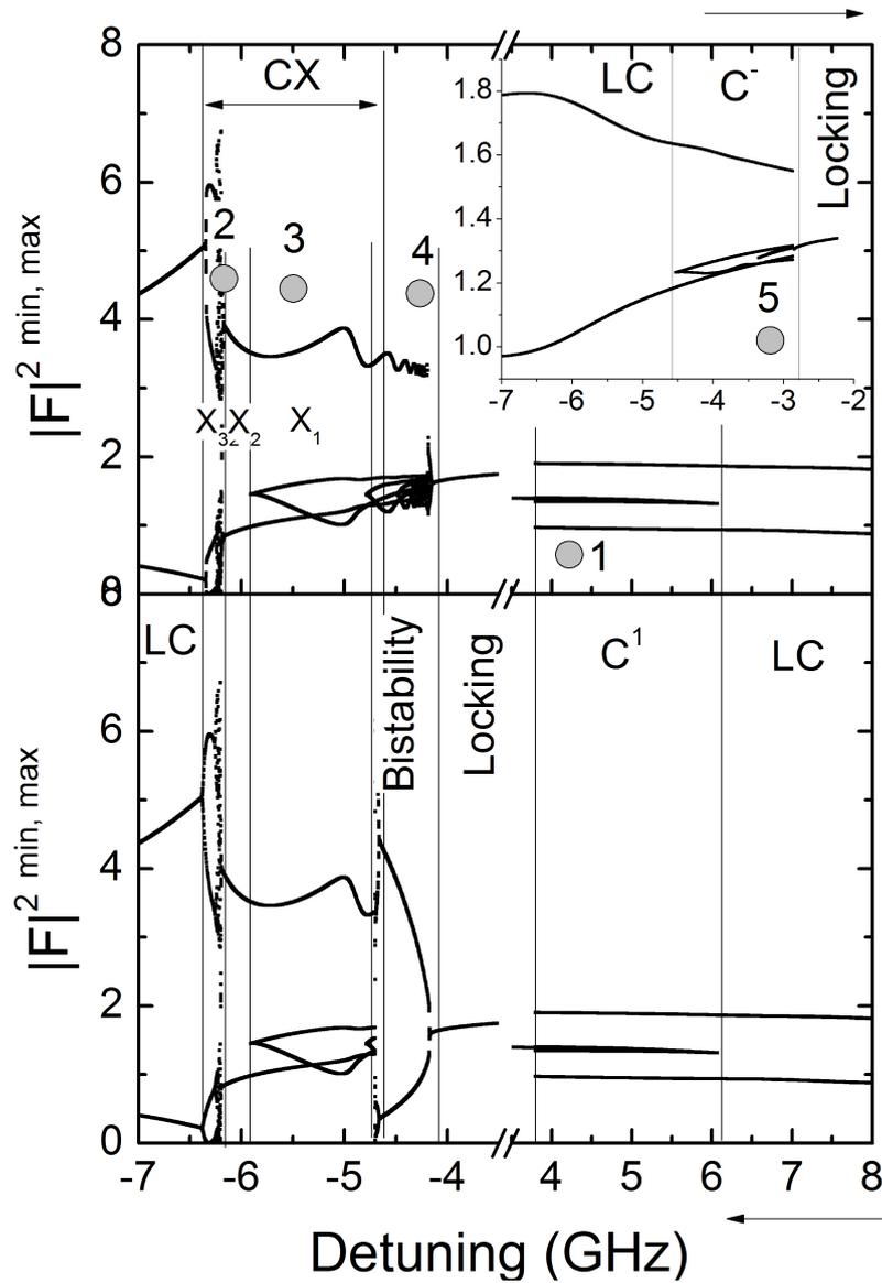
Figure 4.13: 1-parameter bifurcation diagrams for  $S_m = 10^{-4} \text{ J/m}^3$  (the inset shows bifurcation diagram for  $S_m = 0.5 \times 10^{-4} \text{ J/m}^3$ ) when sweeping the detuning either from negative to positive (top plot) or from positive to negative (bottom plot) values.
