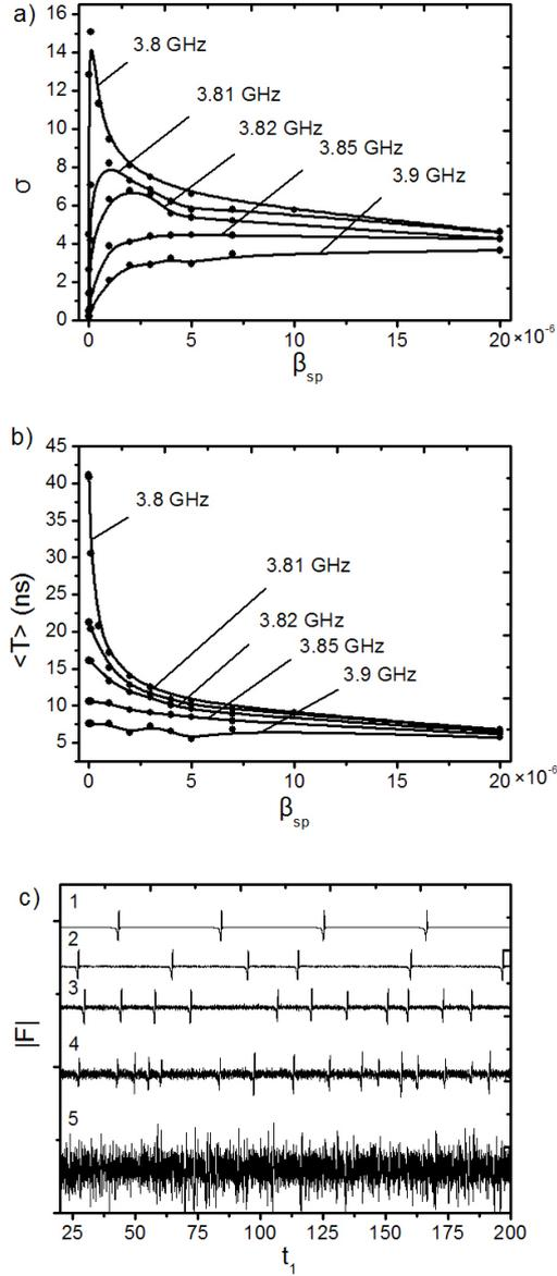
Figure 4.21: a) Standard deviation  $\sigma$  and b) mean  $\langle T \rangle$  of the interpose time distribution as a function of the spontaneous recombination noise strength.  $S_m = 10^{-4} \text{ J/m}^3$ . c) Time traces at the detuning of 3.8 GHz and 1:  $\beta_{sp} = 0$ , 2:  $\beta_{sp} = 10^{-7}$ , 3:  $\beta_{sp} = 10^{-6}$ , 4:  $\beta_{sp} = 5 \cdot 10^{-6}$ , 5:  $\beta_{sp} = 10^{-4}$ .
