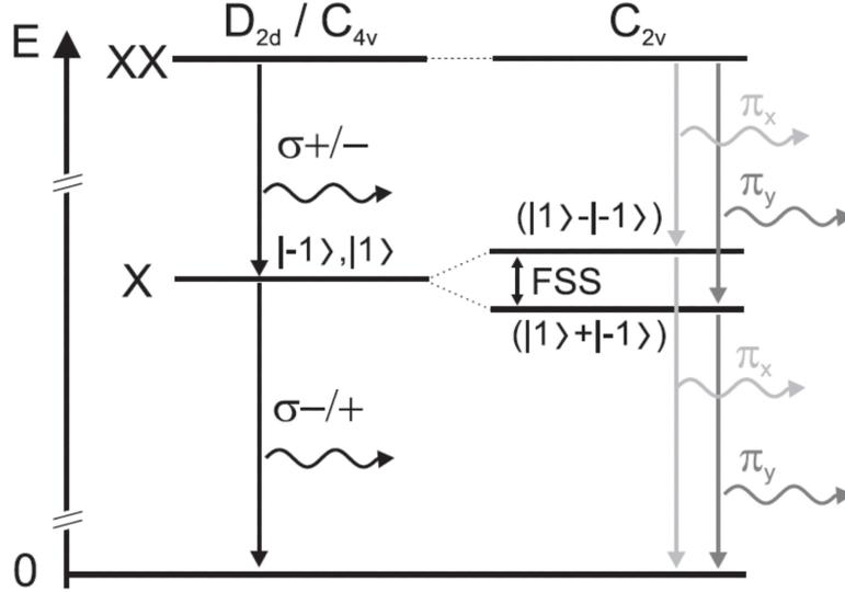
Figure 2.8: Effect of the exchange interaction on the exciton (X) bright states. XX denotes the biexciton ground state.  $|J_z\rangle$  is the exciton total angular momentum,  $\sigma\pm$  denotes circularly polarized light, and  $\pi_{x/y}$  linearly polarized light with  $x = [110]$  and  $y = [1-10]$ .  $D_{2d}$ ,  $C_{4v}$ , and  $C_{2v}$  indicate the confinement potential symmetry. Taken from [129].
