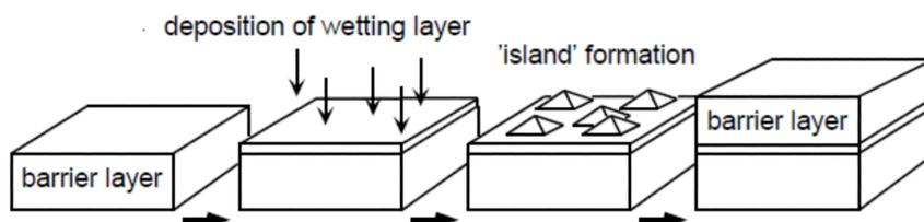
Figure 1.8: Schematic representation of Stranski-Krastanov growth of quantum dots. The QDs (shown as small pyramidal ‘islands’) grow spontaneously from on the deposited wetting layer due to strain relaxation. Taken from [74]
