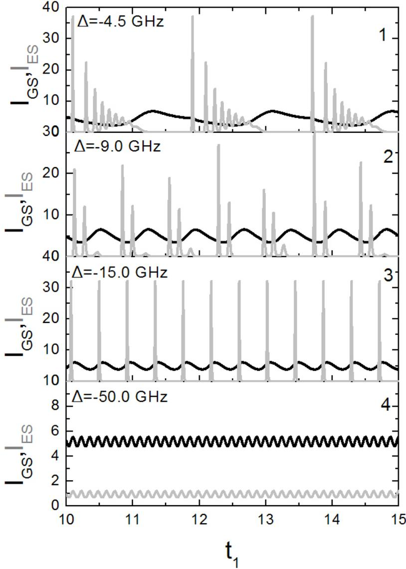
Figure 5.8: Temporal evolution of the *GS* and *ES* mode intensities for  $S_m = 1.5 \times 10^{-4} \text{ J/m}^3$  and 1:  $\Delta = -4.5 \text{ GHz}$ , 2:  $\Delta = -9.0 \text{ GHz}$ , 3:  $\Delta = -15.0 \text{ GHz}$ , 4:  $\Delta = -50.0 \text{ GHz}$ .
