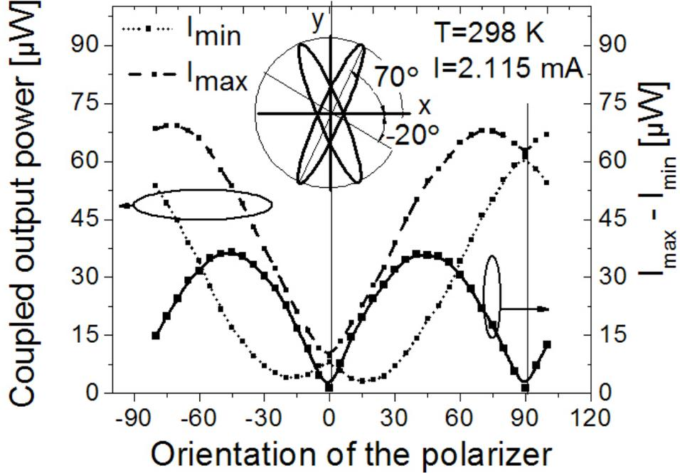
Figure 2.15: Maximum  $I_{max}$  (dashed curve) and minimum  $I_{min}$  (dotted curve) of the output power at the switching as a function of the polarizer direction, measured at a current of 2.115 mA and temperature of 298K. The solid curve shows the difference  $I_{max} - I_{min}$ , i.e. the amplitude of switching. The inset shows the orientation of the determined polarization ellipses between which polarization mode hopping takes place.
