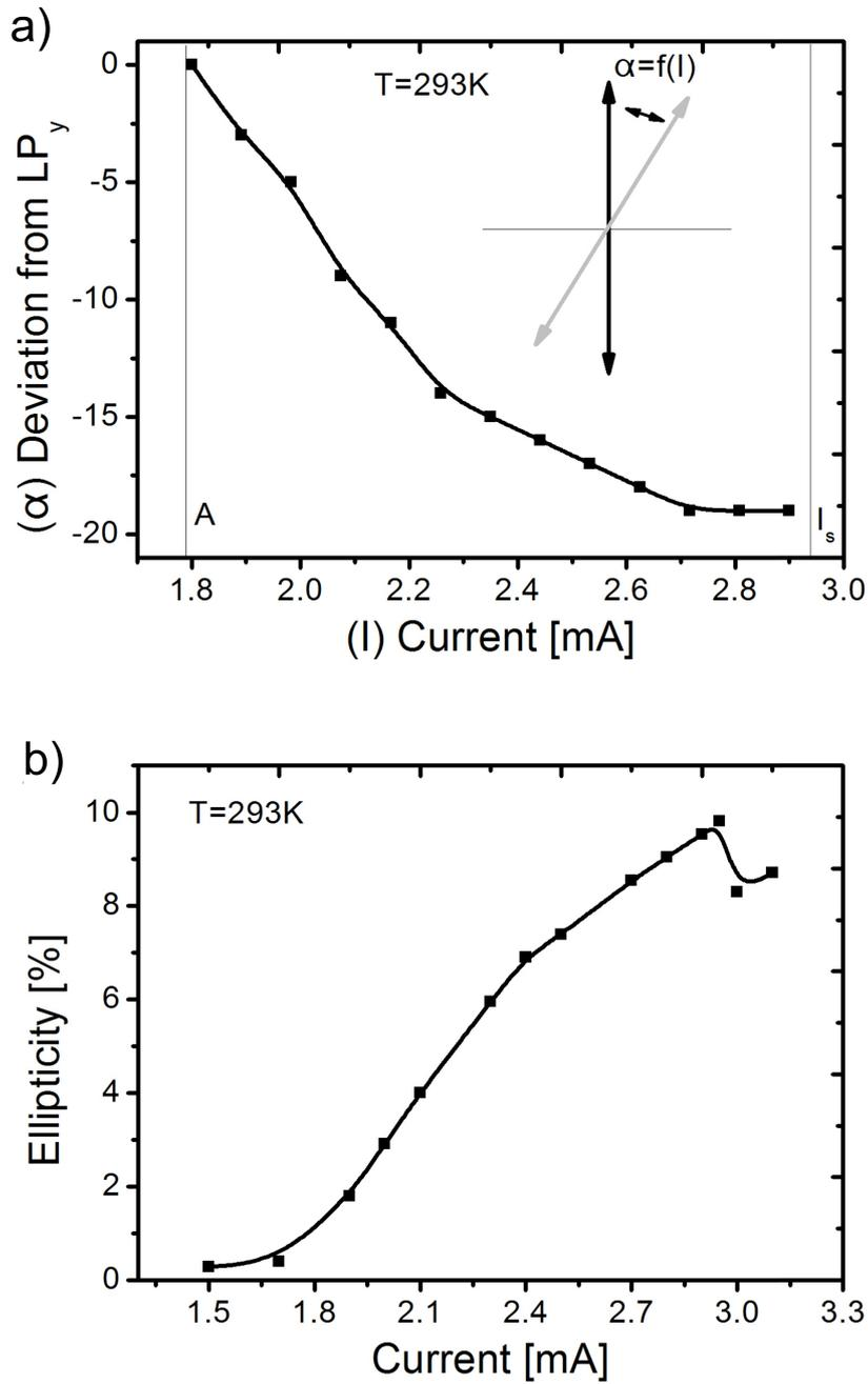
Figure 2.14: a) Current dependence of the angle  $\alpha$  between the orientation of the  $y$ -LP mode and the major axis of the polarization ellipse of the  $EP$  mode. b) Current dependence of the ellipticity of the  $EP$  mode.
