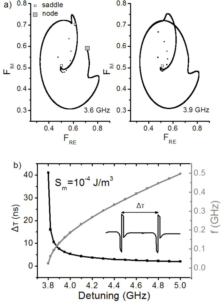
Figure 4.17: a) Phase diagrams for  $S_m = 10^{-4} \text{ J/m}^3$  and  $\Delta = 3.6$  GHz (left),  $\Delta = 3.9$  GHz (right). b) Time difference (and corresponding frequency,  $f$ ) between consecutive pulses in the region  $C^1$  as a function of the detuning.
