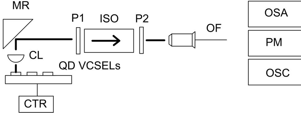
Figure 2.10: Experimental set-up. CTR: current driver and temperature controller, CL: collimator, MR: mirror, P1,P2: polarizers, ISO: optical isolator, OF: optical fiber, OSA: optical spectrum analyzer, PM: power meter, OSC: oscilloscope.
