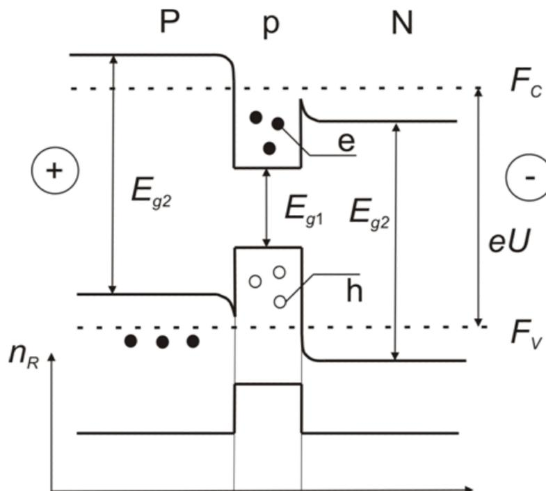
Figure 1.1: Double heterostructure in which a lower energy bandgap material  $E_{g1}$  is sandwiched between materials with larger energy bandgap  $E_{g2}$ , which leads to both optical and carrier confinement, the former due to larger refractive index  $n_R$  of materials with narrower energy bandgap.
