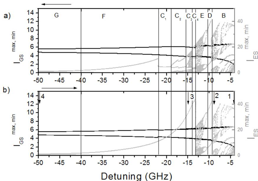
Figure 5.7: 1-parameter bifurcation diagram for  $J = 17$ ,  $S_m = 1.5 \times 10^{-4} \text{ J/m}^3$  for detuning when sweeping the detuning either from a) small to large or b) from large to small negative values. Arrows 1-4 correspond to time traces in Fig. 5.8-1:4.
