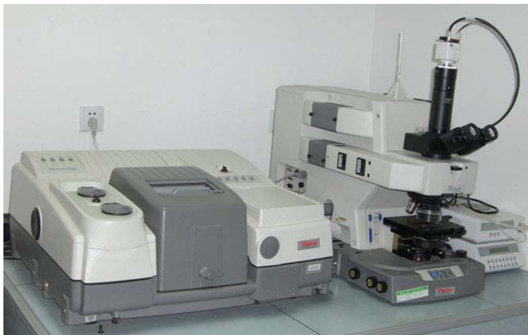
Fig. 4- 1 Picture for the Nicolet 5700 FTIR spectrometer coupled with a microscope
