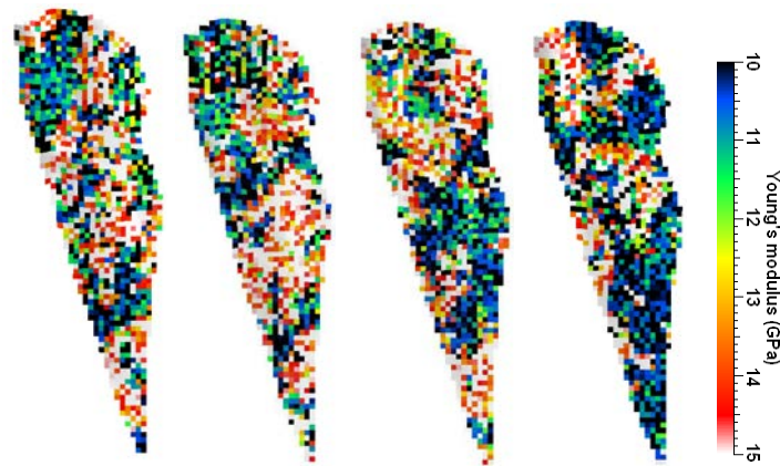
Figure 6: Realizations of the Young's modulus of the layer within the Ness associated to the lithofacies simulations displayed on Figure 5
