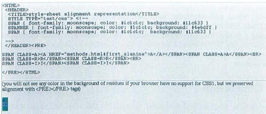
Figure 8: Cascade Style Sheet MSA representation with hyper-links.
