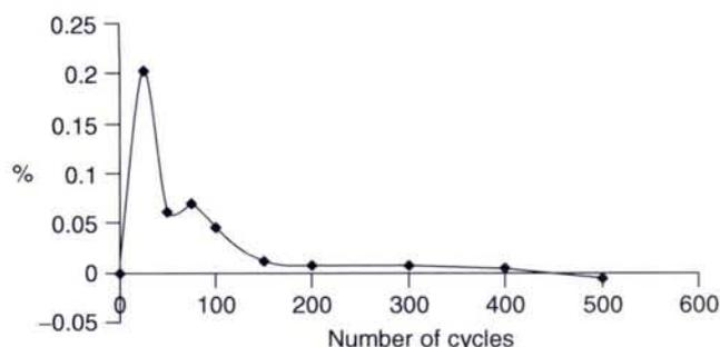
**Figure 2.** Experimental intensity of the longitudinal two-spin order (in percent, relative to equilibrium magnetization) created by the double train of  $\pi$  pulses, as a function of the number of cycles (50 ms between consecutive pulses).
