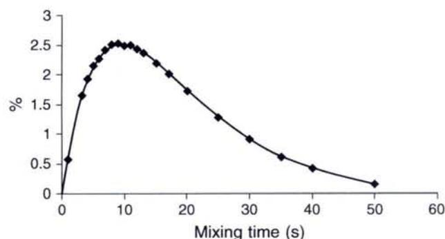
**Figure 8.** Experimental data (dots) obtained on  $^{13}\text{C}$ -labeled formic acid (degree of labeling: 99%) at ambient temperature with the sequence of Fig. 7 (Bruker DRX spectrometer operating at 9.4 T; proton resonance frequency: 400 MHz). These data represent the intensity of the longitudinal two-spin order as a function of the mixing time. The theoretical curve has been calculated with the parameters given in the legend to Fig. 3.
