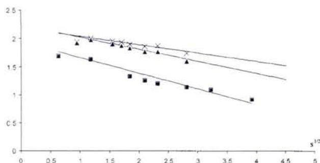
FIG. 3. Proton experimental data presented according to Eqs. (11) and (12):  $[1 - S(\Delta)/S_0]/e^{-\Delta/T_1}$  as a function of  $\Delta$ . Crosses: ethanol. Triangles: water. Squares: acetone. Same parameters for slice selection as in Fig. 2.
