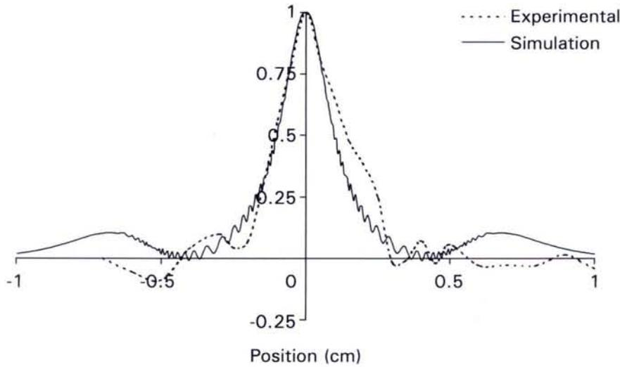
**Fig. 2.** Comparison of experimental and simulated profiles corresponding to a slice selection obtained with the S<sup>2</sup>P sequence for  $\tau = 0.1$  s,  $n = 100$  ( $T_1 = T_2 = 3$  s,  $T_2^* = 0.05$  s). The shoulder at the right part of the experimental trace is again due to the same type of imperfections as those mentioned in Fig. 1 (results of Figs. 1 and 2 have been obtained with different test samples).
