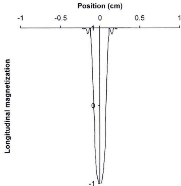
FIG. 1. Profile of the longitudinal magnetization (simulation performed according to methods developed in Ref. 4) corresponding to the application of sequence (15) with  $n\alpha = \pi$ . For this simulation, the  $B_1$  field profile was assimilated to a Gaussian function (in view of experimental determination of the actual amplitude of  $B_1$  along the considered axis) with a standard deviation of 1.5 mm and  $n$  was set at 64.
