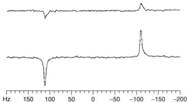
**Figure 6.** Experimental results obtained on pure  $^{13}\text{C}$ -labeled formic acid (degree of labeling: 99%) with the sequence of Fig. 5 for two different mixing times: 2 s (top) and 12 s (bottom). Experiments performed at ambient temperature with a home-made spectrometer ( $^1\text{H}$ : 200 MHz); 64 scans were accumulated. The temperature of the sample was kept constant by an air flow.
