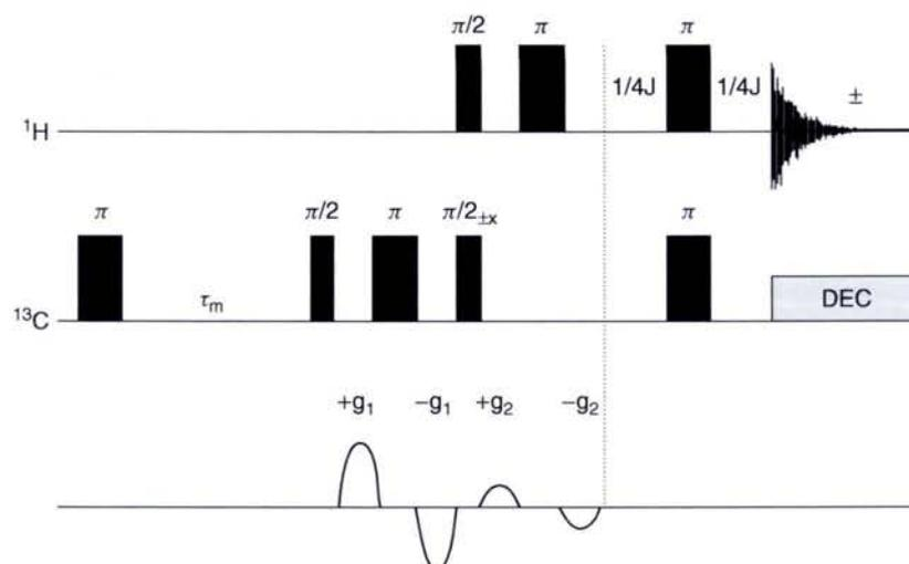
**Figure 7.** The homologous sequence of the one in Fig. 5 with static field gradient pulses. Bipolar gradients are used (for improving the experiment quality) with  $g_1/g_2 = \gamma_H/\gamma_C$ . The phase cycling has the same purpose as that indicated in Fig. 5. At the level of the dotted vertical line, only the antiphase doublet exists. It can be (optionally) refocused by the sub-sequence displayed on the right of the dotted vertical line.
