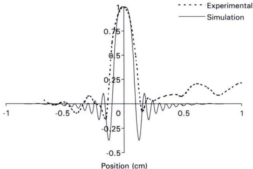
**Fig. 1.** Comparison of experimental and simulated profiles corresponding to a slice selection obtained with the DANTE-like sequence for  $n = 10$ . The horizontal scale corresponds to the axis of the rf coil, the origin coinciding with the coil center. The right part of the experimental trace involves an unwanted signal due to imperfections of the experimental device.
