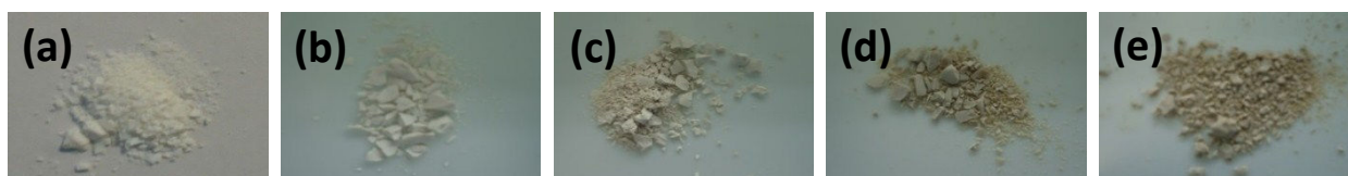
Fig. 3.2.2. Photographs showing the color change of Cu/ZIF-8 crystals upon increasing the doping percentage in copper. (a) ZIF-8 as reference, (b), (c), (d) and (e) are ZIF-8 crystals doped with 0.6, 2.1, 3.9 and 8.7% Cu, respectively.
