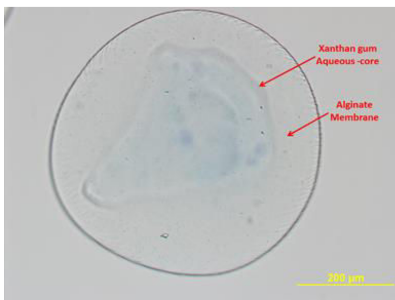
Figure 29: Microscopic image of single alginate-xanthan gum microcapsule
