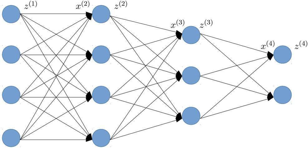
Figure 8.2: Model of a multilayer perceptron with four layers: input, two hidden layers and output layer.
