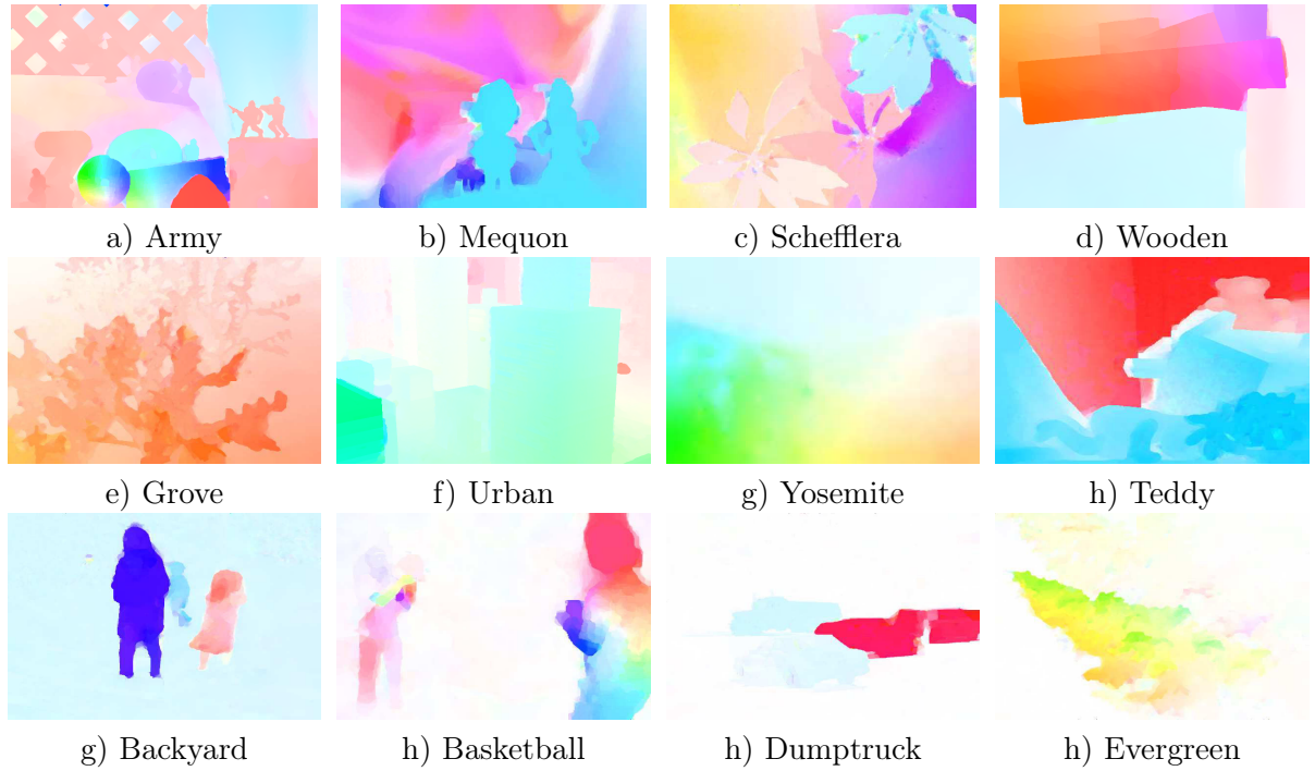
Figure 4.8: Optical flow results (in flow color code) obtained with the proposed method ( ROF-NND ) for the Middlebury test dataset (hidden ground truth).
