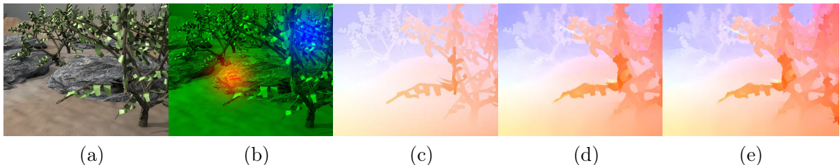
Figure 4.1: Visualization of the robustness of the proposed ROF-NND method against illumination changes. (a) Original frame 10 of Grove3. (b) Frame 11 of Grove3 with illumination. (c) Ground truth flow. (d) Result with ROF-NND before illumination changes ( AEPE/AAE = 0.58/6.05 ). (e) Result of ROF-NND after illumination changes ( AEPE/AAE = 0.58/6.05 ).
