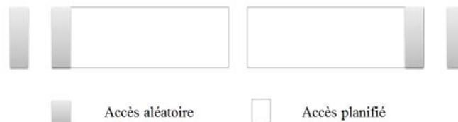
Figure 17 : Protocole TRAMA (*Traffic Adaptive Medium Access Control*)
