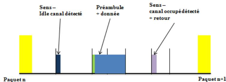
Figure 28 : Protocole PSMA (*Preamble Sense Multiple Access*)
