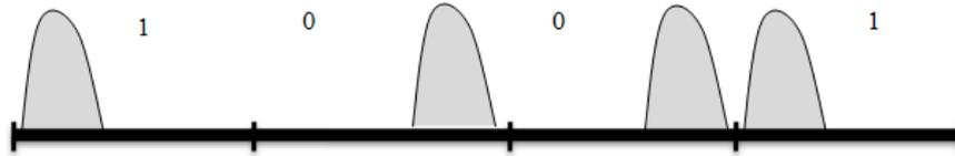
Figure 36 : Modulation PPM
