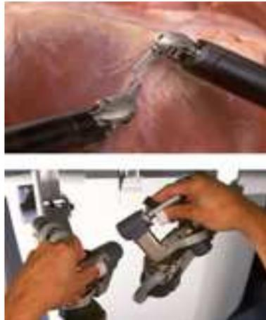
**FIGURE 1.2.** Instruments du robot (Intuitive Surgical ©)
