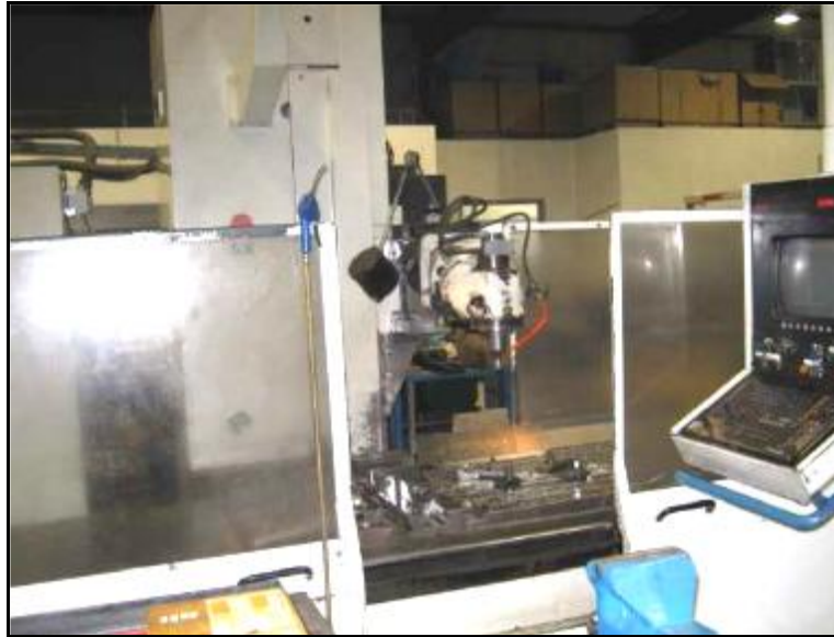
Figure 3.3. Centre de fraisage Huron SX 523.
