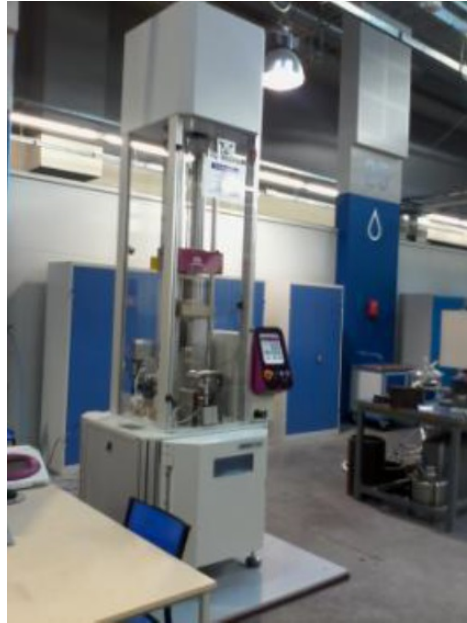
FIGURE 3.19 – Tour de chute CEAST 9350.
