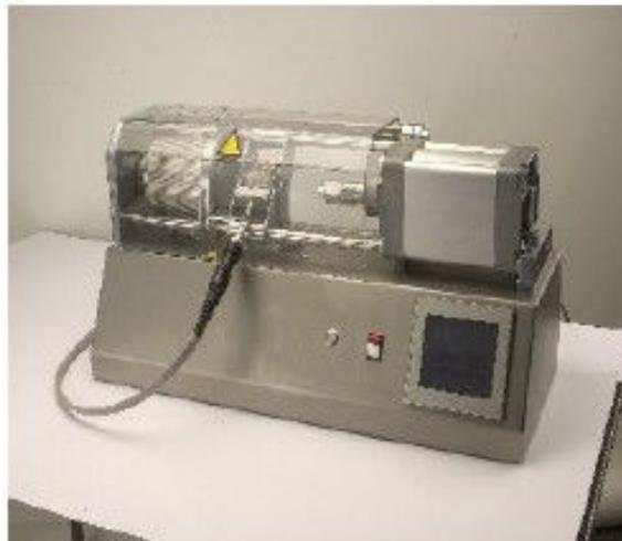
Figure 2.5 - Mini-injection molding.
