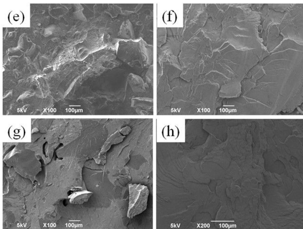
Figure 4.8 - SEM photographs of the fracture surfaces of the original GTR/PS blends and GTR-g-PS/PS blends. The equivalent GTR content is 16%, 22%, 30% and 38% from top to bottom. The original GTR/PS blends are a, c, e, and g, and the GTR-g-PS/PS blends are b, d, f, and h.
