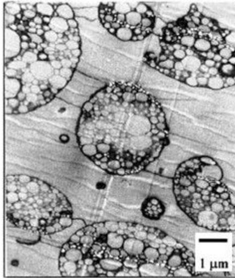
Figure 1.4 - Salami structure of high-impact polystyrene [48].
