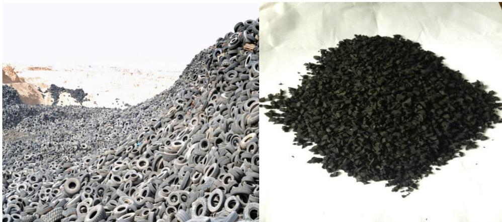
Figure 1.3 - Waste tire and ground tire rubber (GTR).
