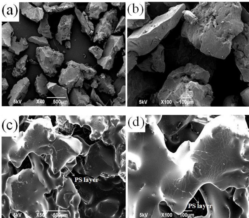
Figure 4.16 - SEM micrographs of original GTR particles and GTR-g-PS particles. The original GTR particles are a and b, and the GTR-g-PS particles are c and d.
