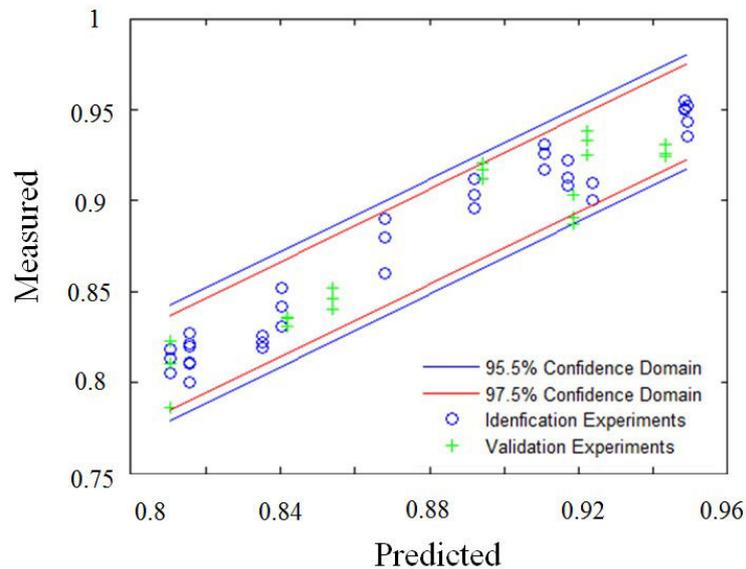
Figure 4.29 - Student test for conversion of styrene.
