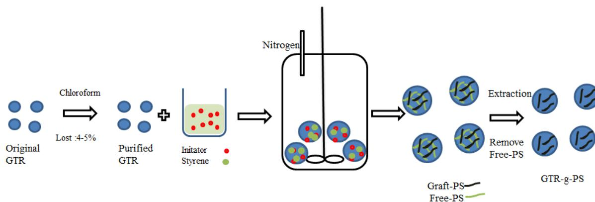
Figure 2.2 - A process of the polymerization of styrene inside GTR particles.
