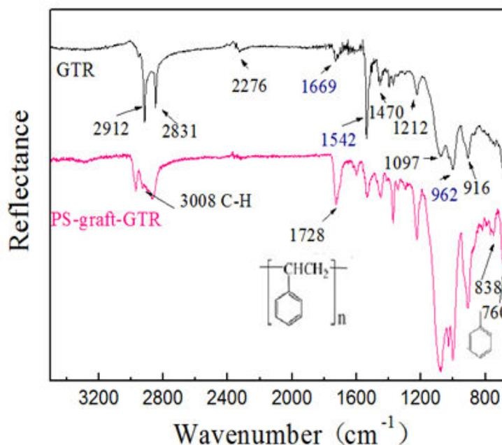
Figure 4.2 - FTIR of GTR particles and GTR-g-PS particles.
