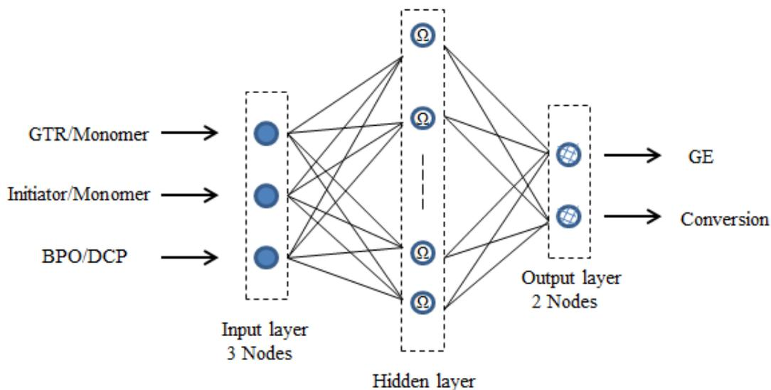
Figure 1.9- Architecture of neural network model.
