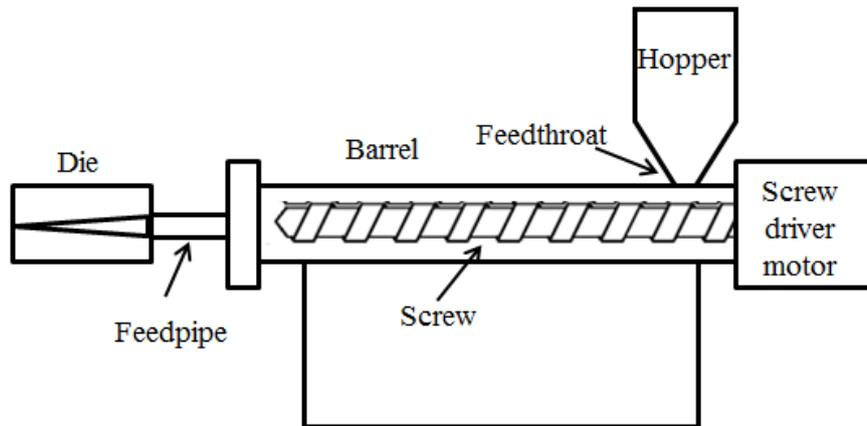
Figure 1.5 - A scheme of a screw extruder.
