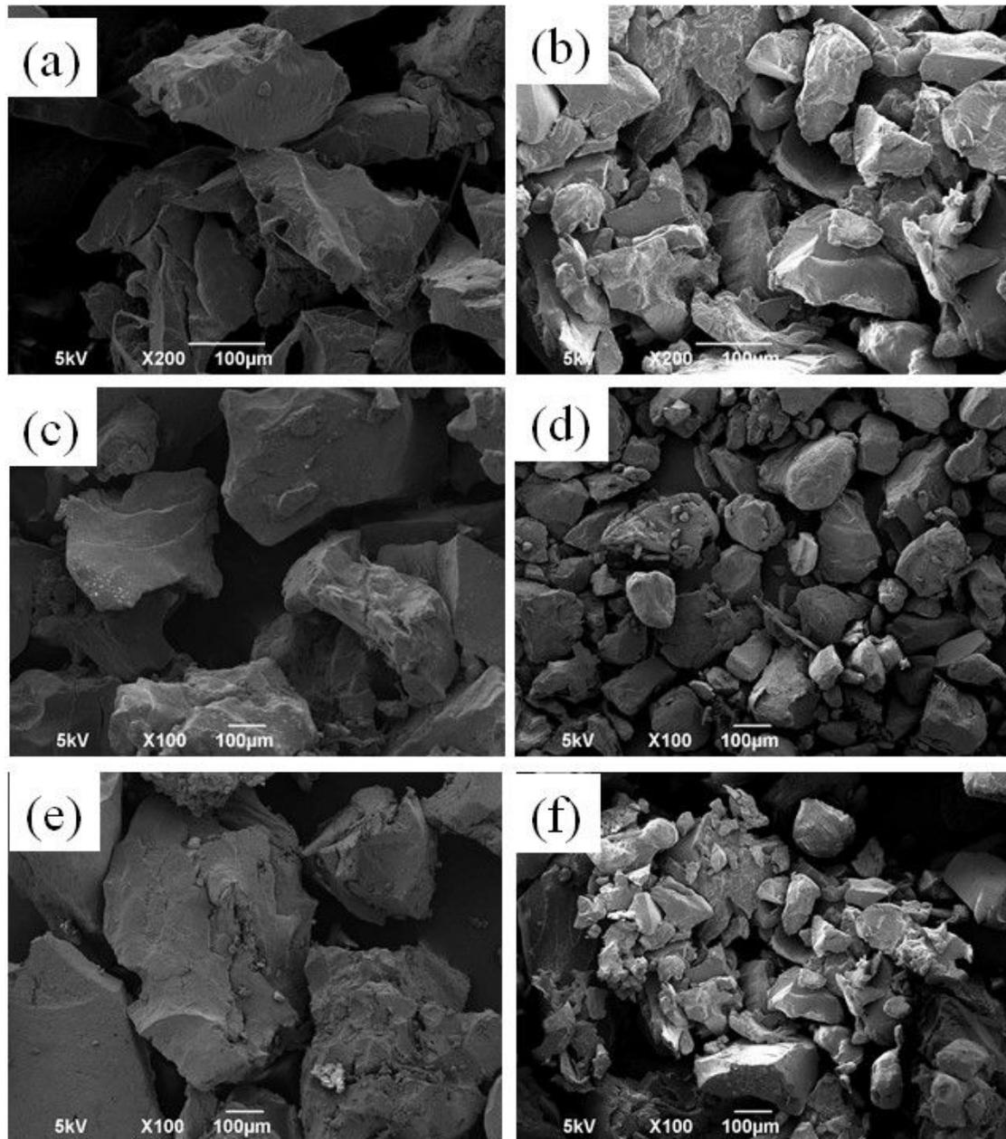
Figure 4.9 - SEM micrographs of the original GTR particles and GTR-g-PS ones. The equivalent GTR content is 16%, 30% and 38% from top to bottom. The original GTR particles are a, c, and e, and the GTR-g-PS particles are b, d, and f.
