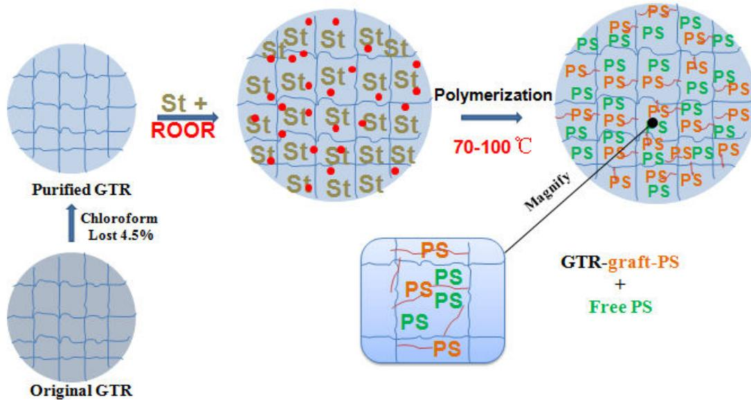
Figure 2.1- A scheme of the polymerization of styrene inside a single GTR particle.
