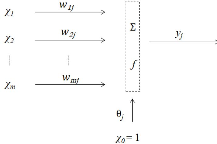
Figure 1.8 - Diagram of one neuron (node).
