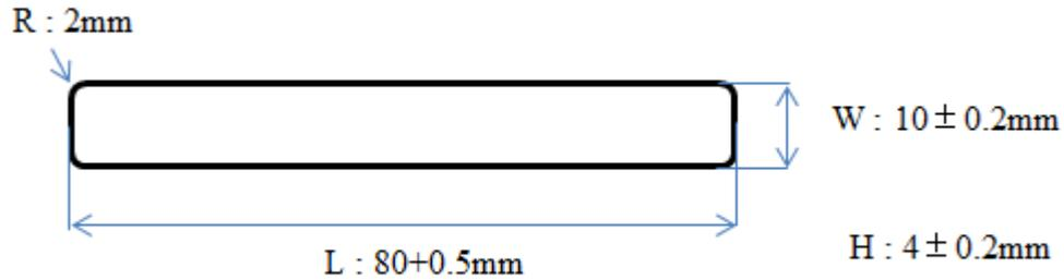
Figure 2.6 - Injection molding of specimens for impact testing.
