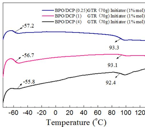
Figure 4.20 - Effect of BPO/DCP on the glass transition temperature of GTR-g-PS particles.
