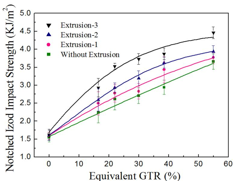
Figure 4.11 - Impact strength of the GTR-g-PS/PS blends after 1, 2 and 3 times of extrusion in a twin screw extruder of type PTW 24. The equivalent GTR content is 16, 22, 30, 38 and 55, respectively.
