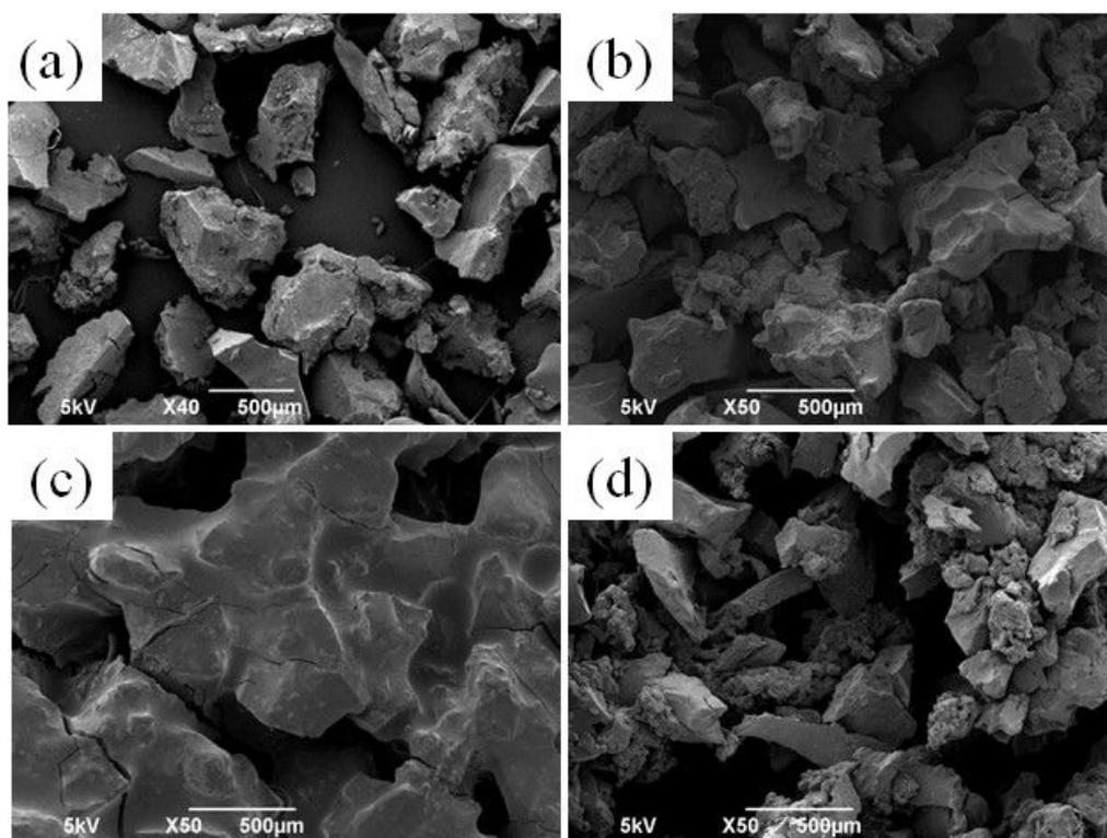
Figure 4.1 - SEM photographs of the original GTR (a), purified GTR (b), GTR-g-PS+Free-PS (c) and GTR-g-PS (d) particles.
