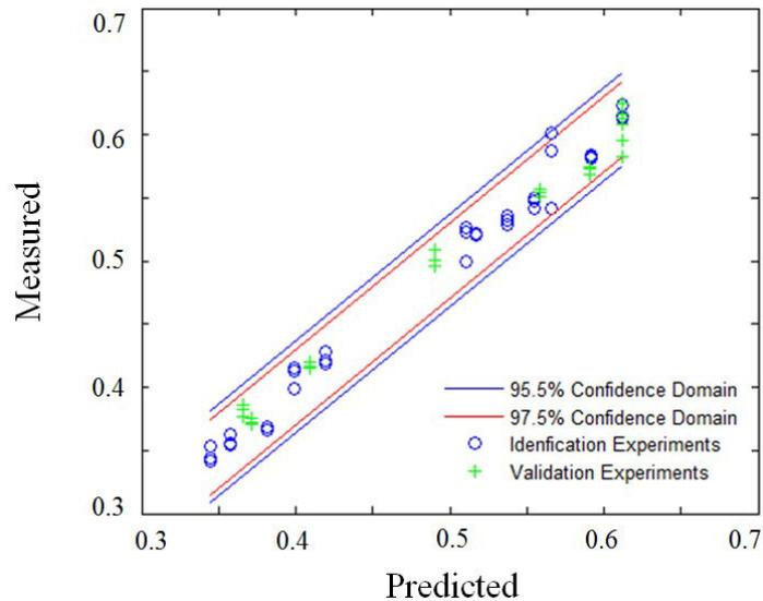
Figure 4.30 - Student test for GE of styrene.
