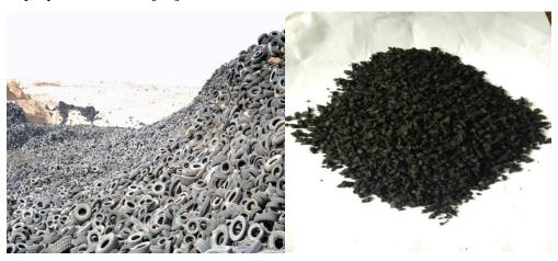
Figure 1.3 - Waste tire and ground tire rubber (GTR).
