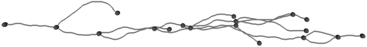
Figure 8: Karst network simulation showing uncontrollable intersections and overlappings. The grey spheres are located where the reconnections between conduits are controlled, and every conduits crossings without a sphere are uncontrolled. This uncontrollability leads sometimes to networks with bad shapes and geologic unlikelihood.
