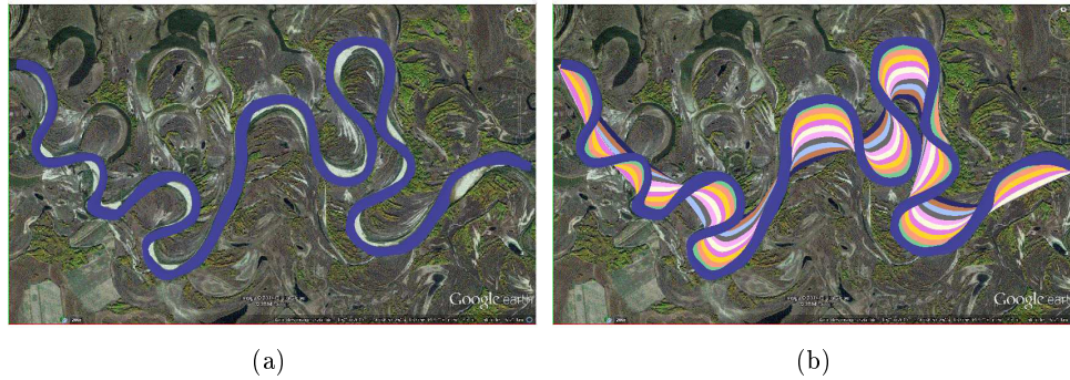
FIGURE 4.10 – MODELING OF AN OPTIMIZED CHANNEL’S POINT BARS USING A RETRO-MIGRATION PROCESS INSPIRED BY THE MIGRATION PROCESS PRESENTED BY RUIU et al. [2014A]. (A) OPTIMIZED CHANNEL ON THE SONSHUA RIVER [GOOGLE EARTH, OCTOBER,10 2010]. (B) POINT BARS WITH THE RETRO MIGRATION PROCESS (10 STEPS).. Modeling of an optimized channel’s point bars using a retro-migration process inspired by the migration process presented by Ruiiu et al. [2014a]. (a) Optimized channel on the Sonshua river [Google Earth, October,10 2010]. (b) Point bars with the retro migration process (10 steps).
