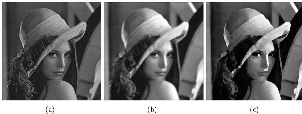
FIGURE A.1 – IMAGE PRE-PROCESSING. (a) Original image. (b) Gaussian Filter. (c) Kuwahara filter.
