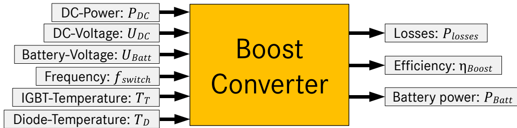
Figure 62: Component behavior modeling approach for a boost-converter
