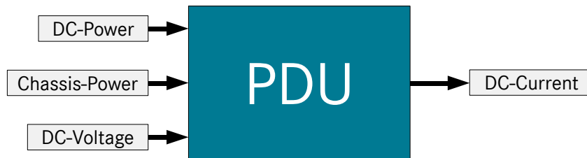
Figure 127: Modeling approach of the power distribution unit
