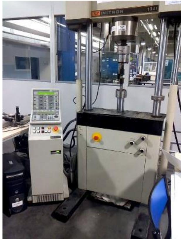
**Figure II.10 :** Machine de traction/compression Instron
