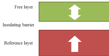
Figure I.4: Schematic of a perpendicularly magnetized tunnel junction with the free layer in green and the reference layer in red.
