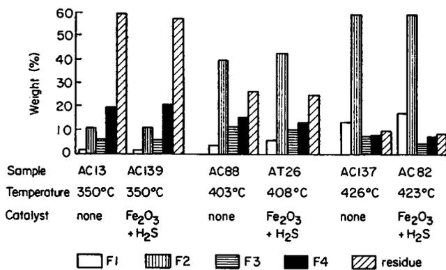
Figure 4 Comparison of hydroliquefaction products
