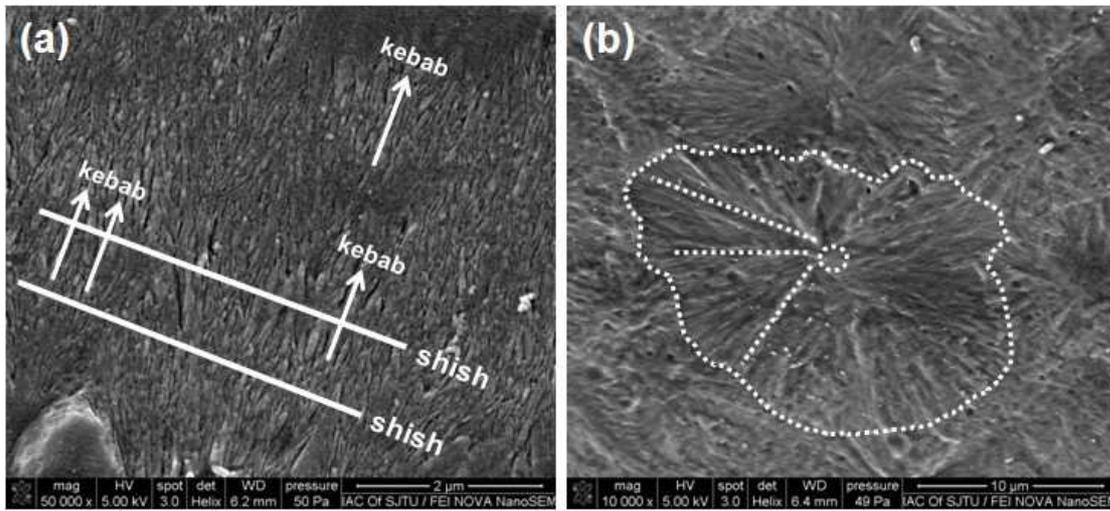
Fig. 4.5 SEM photographs of the injection-molded iPP samples after etching. (a) skin layer, and (b) core layer.
