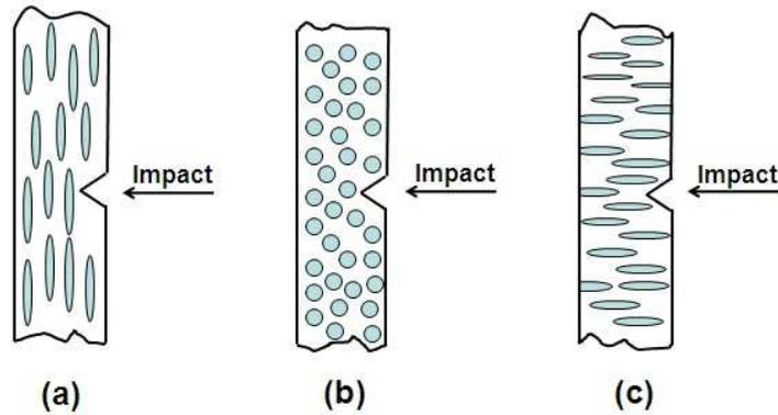
Fig. 5.16 The schematic representation of the relation between the bubbles orientation and the fracture propagation direction. (a) c-oriented bubbles, (b) isotropy bubbles, (c) a or b-oriented bubbles.
