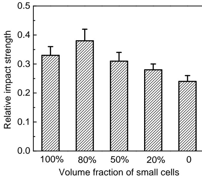
Fig. 6.14 The notched impact strength bi-modal cell structure foams with different volume fraction of small cells. The relative densities of the samples are all about  $0.3\pm 0.02$ . The cell size of large cells is  $100\pm 12\ \mu\text{m}$ , and the cell size of small cells is  $10\pm 1.5\ \mu\text{m}$ .
