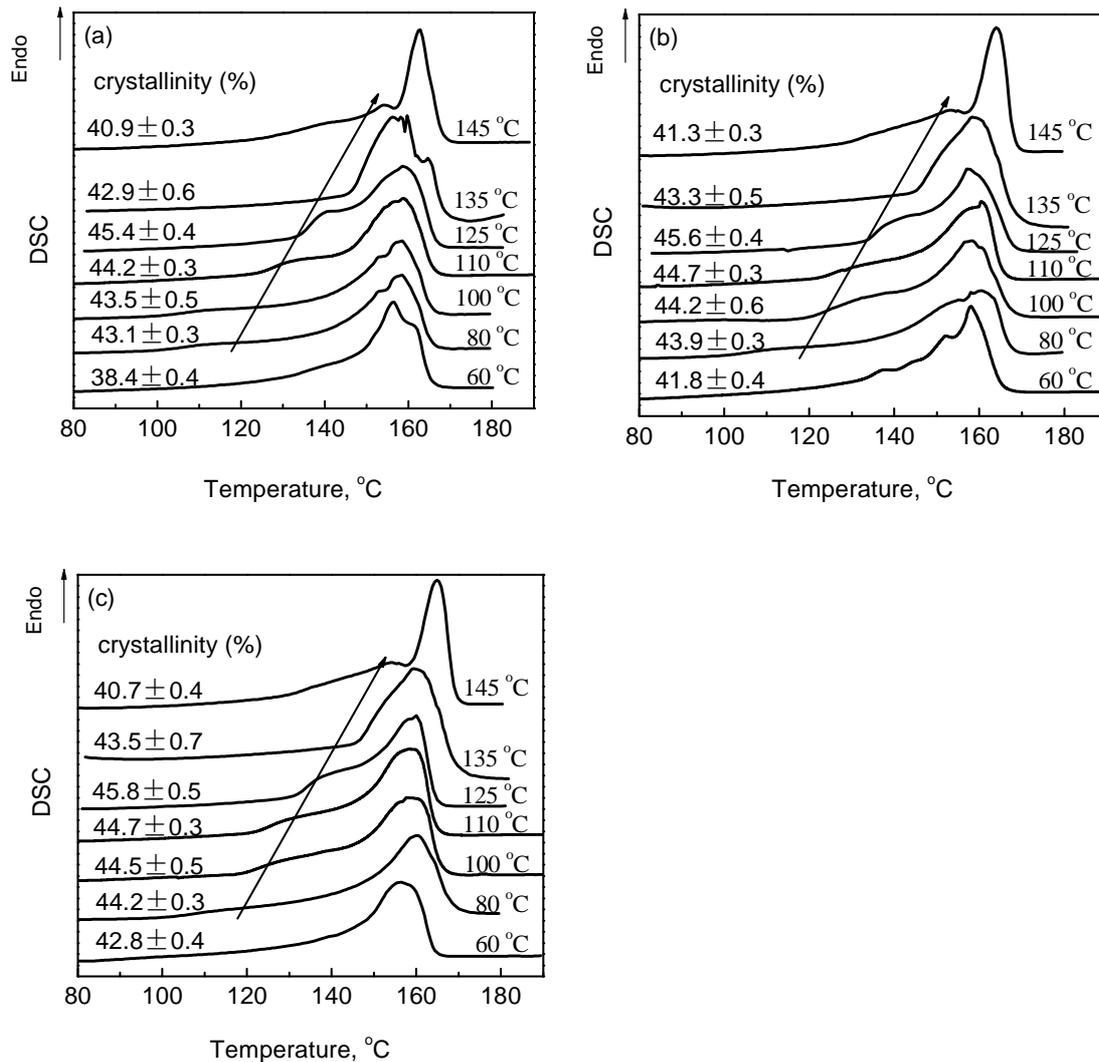
Fig. 3.15 DSC thermograms of PP2 treated under 15MPa CO<sub>2</sub> pressure and various temperature (60, 80, 100, 110, 125, 135, 145°C), in (a) the skin layer, (b) the intermediate layer and (c) the core layer, respectively.
