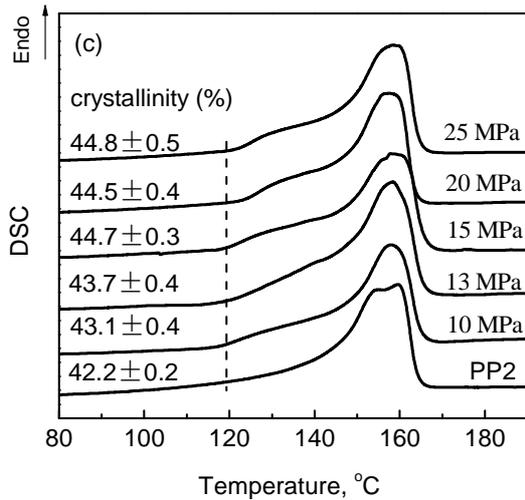
Fig. 3.14 DSC thermograms of PP2 treated under 100°C and various CO<sub>2</sub> pressures (0, 10, 13, 15, 20, 25MPa), in (a) the skin layer, (b) the intermediate layer and (c) the core layer, respectively.
