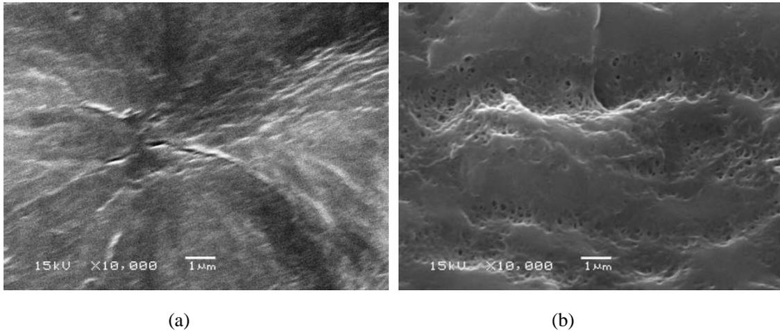
Fig. 4.8 SEM photographs of the skin layer foamed at (a) 115°C and (b) 125°C with a CO<sub>2</sub> saturation pressure of 15 MPa.
