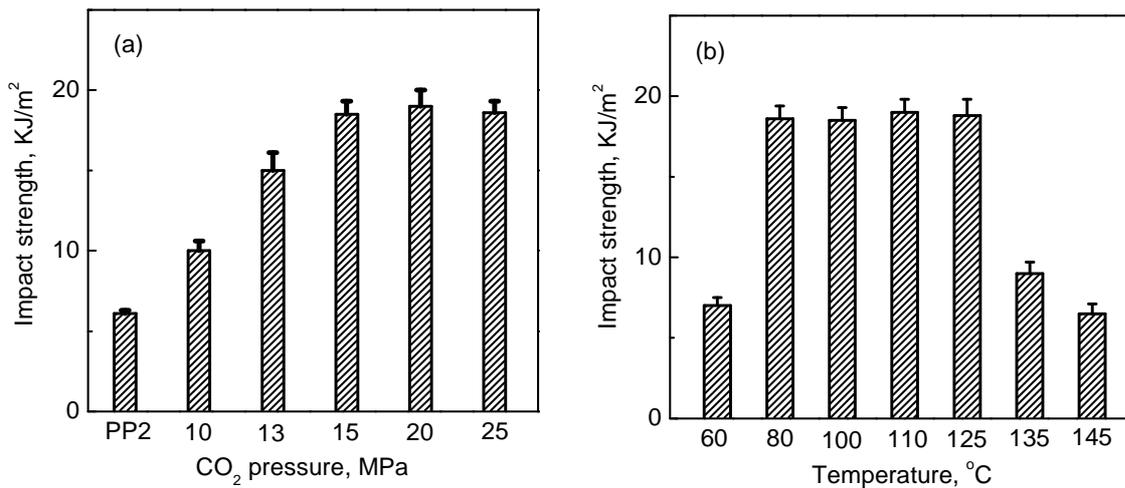
Fig. 3.13 Impact strength of PP2 treated under (a) 100°C and various CO<sub>2</sub> pressures; and (b) 15MPa and various temperatures.
