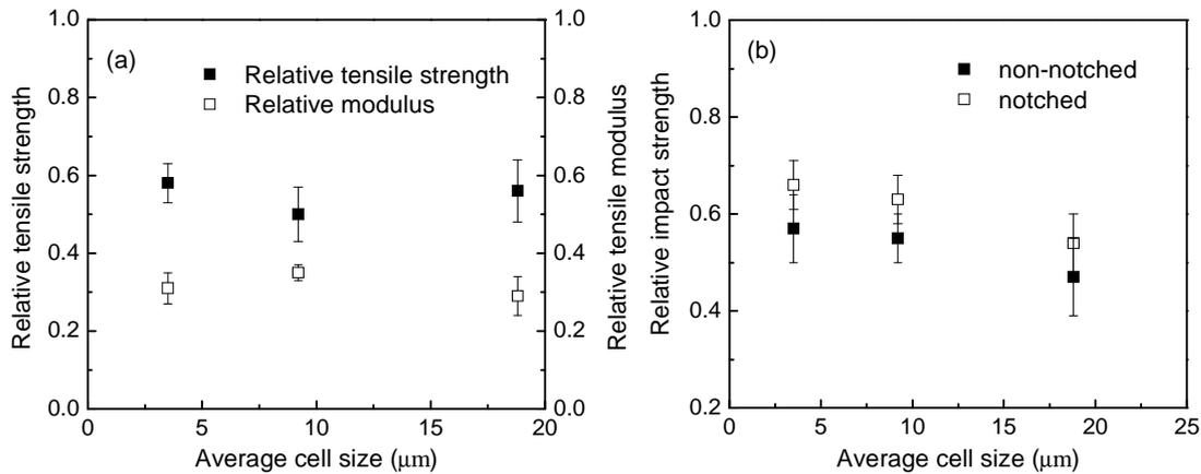
Fig. 5.9 Effect of cell size on mechanical properties in terms of (a) relative tensile strength and relative tensile modulus, and (b) non-notched impact strength and notched impact strength. The relative density is  $0.56 \pm 0.04$ .
