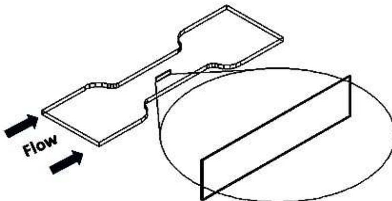
Fig. 2.4 Schematic of the positions of iPP samples for optical light microscopy
