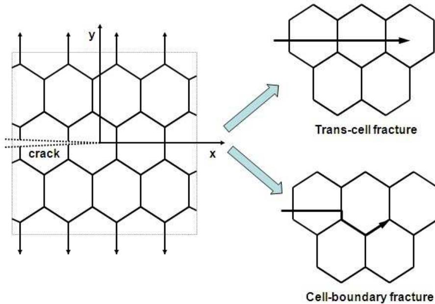
Fig.5.10 Schematic of crack propagation through the bubbles.
