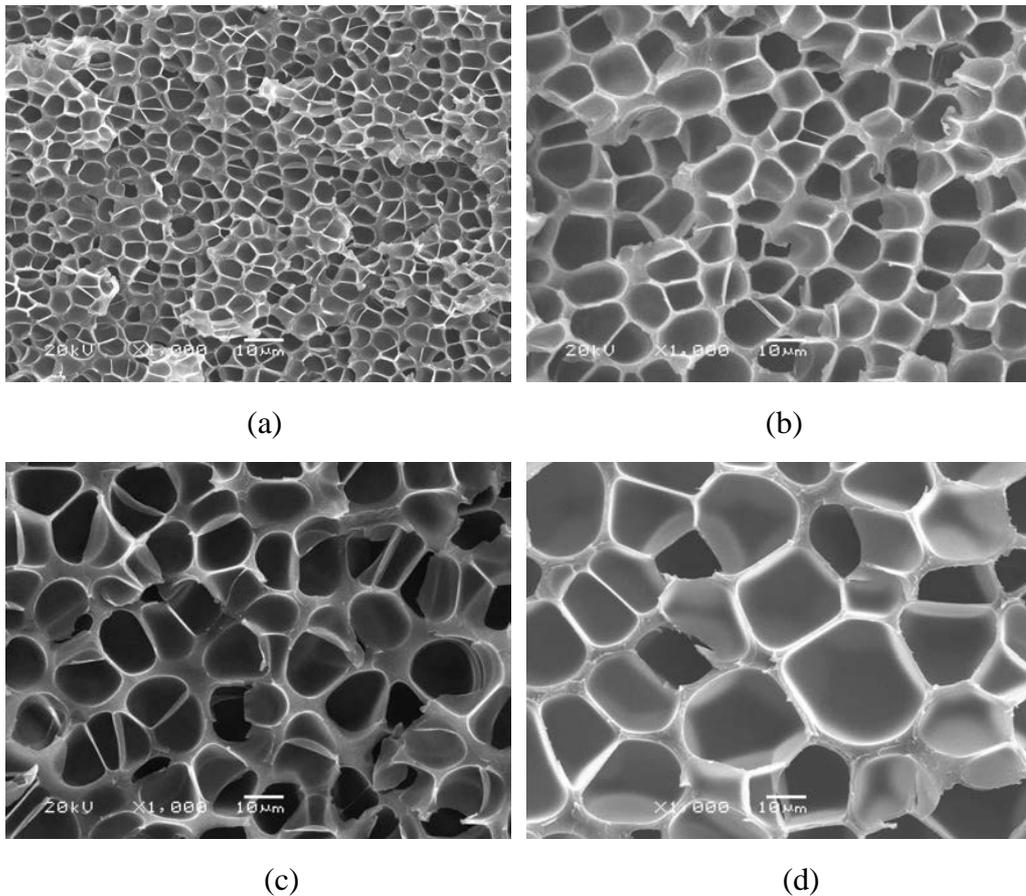
Fig. 5.6 SEM images of cell morphologies of PS foamed in the similar relative density of  $0.3\pm 0.02$  with various average cell size: (a) 6.7  $\mu\text{m}$ , (b) 10  $\mu\text{m}$ , (c) 14.5  $\mu\text{m}$  and (d) 22.5  $\mu\text{m}$ . The white bar is 10  $\mu\text{m}$ .
