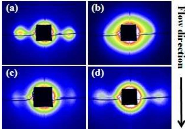
Fig. 3.7 2D SAXS images of (a) PP2 before CO<sub>2</sub> treatment, (b) PP2 after CO<sub>2</sub> treatment, (c) PP1 before CO<sub>2</sub> treatment and (d) PP1 after CO<sub>2</sub> treatment.
