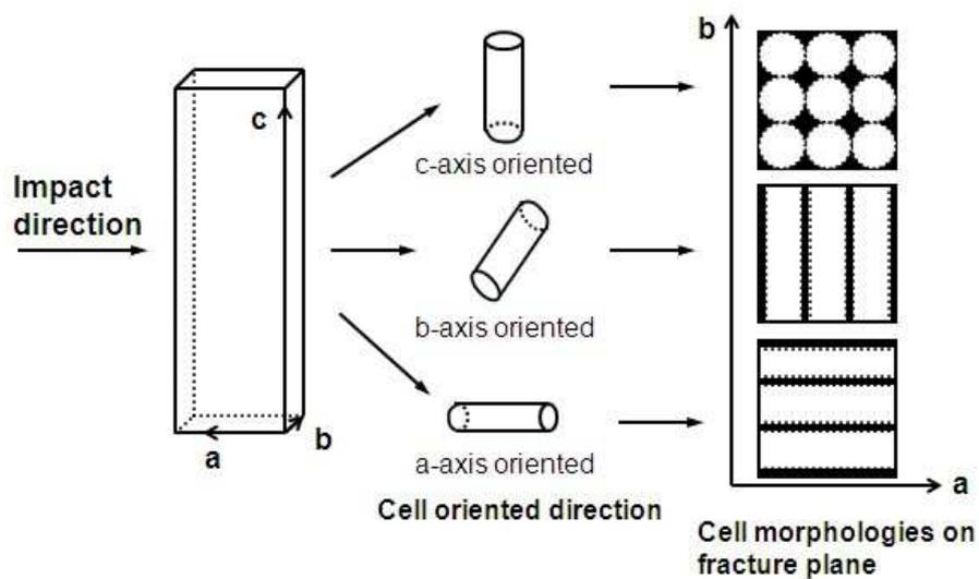
Fig. 2.3 Schematic of cell oriented growth in the mould during the confined foaming.
