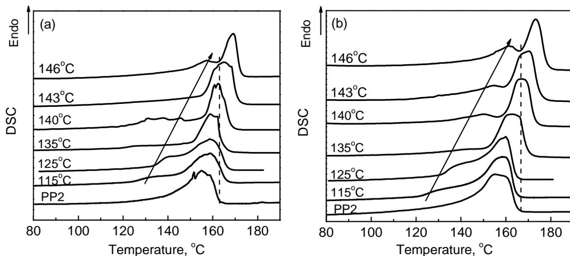
Fig.4.15 DSC thermograms of the skin and core and their foams obtained at 115, 125, 135, 140, 143 and 146 °C, respectively. The saturation CO<sub>2</sub> pressure is 15 MPa. (a) skin, and (b) core.
