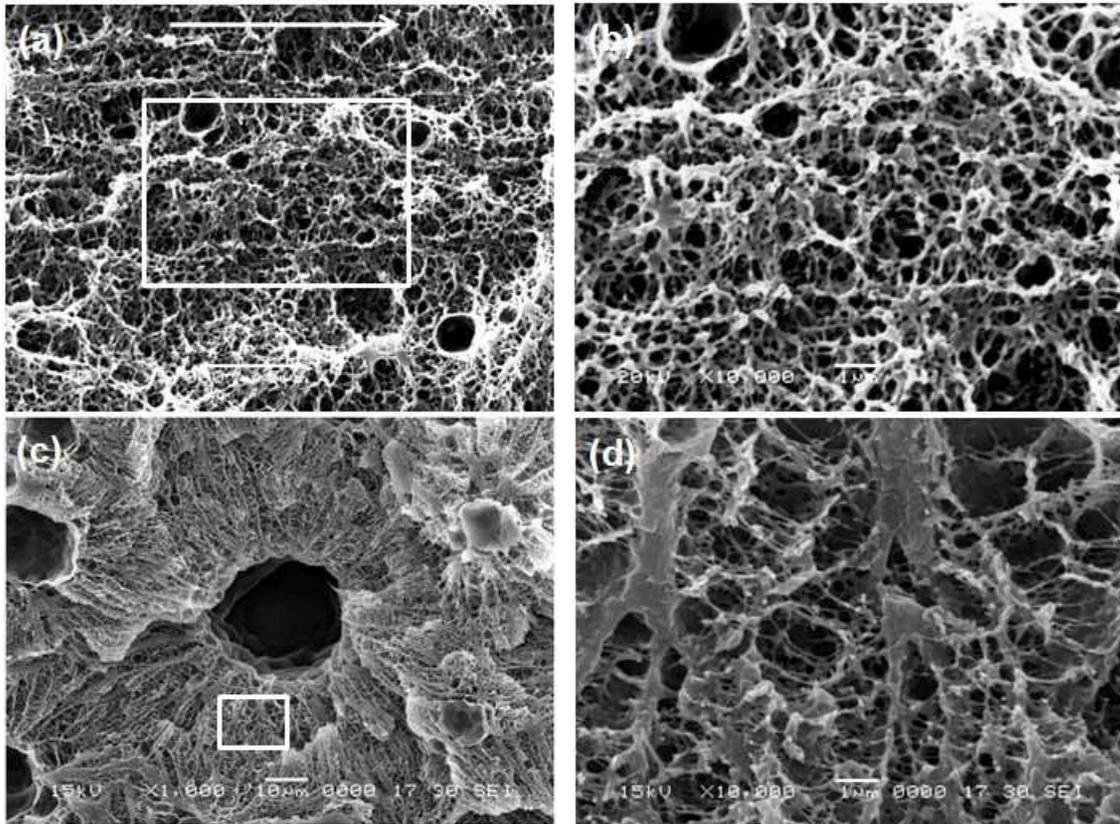
Fig. 4.11 SEM photographs of the skin and core layers foamed at 143 °C and a CO<sub>2</sub> pressure of 15 MPa. (a) skin foam (The white bar is 5 μm and the white arrow indicates the flow direction); (b) magnification of the white rectangle in part (a) (The white bar is 1 μm); (c) core foam; (d) magnification of the white rectangle in part (c).
