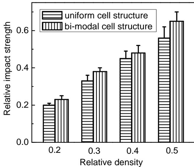
Fig. 6.16 The notched relative impact strength of bi-modal cell structure foams and uniform cell structure foams as a function of relative density. The  $f_s$  of bi-modal foams are all 80%. The average cell size of foams with uniform cell structure is 10  $\mu\text{m}$ . The average cell size of large cells in the bi-modal foams is  $100 \pm 12 \mu\text{m}$ , and the cell size of small cells in the bi-modal foams is  $10 \pm 1.5 \mu\text{m}$ .
