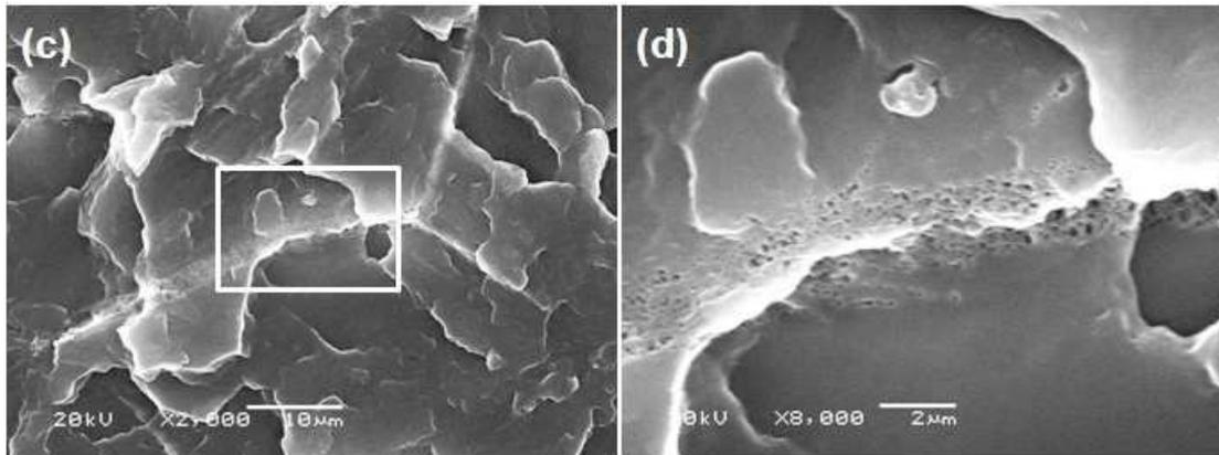
Fig. 4.9 SEM photographs of the skin and core layers foamed at 135 °C and a CO<sub>2</sub> saturation pressure of 15 MPa. (a) skin (the white arrow indicates the flow direction); (b) magnification of the white rectangle in part (a) and the white bar is 1 µm; (c) core; and (d) magnification of the white rectangle in part (c).
