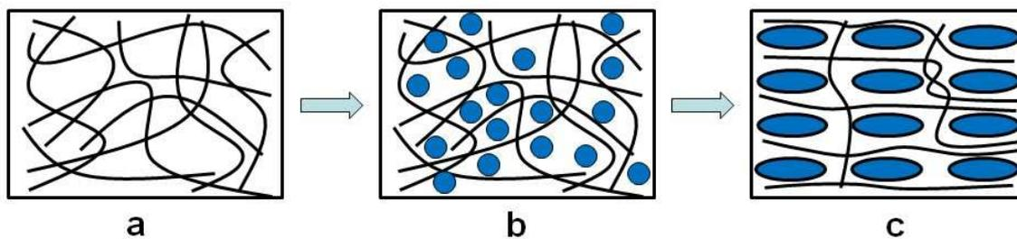
Fig. 5.18 Schematic of molecular chains oriented by the shearing of bubbles growth along the oriented direction: (a) the entangled network with the saturation of  $\text{CO}_2$ ; (b) the cell nucleation and growth between the molecular chains after the gas depressurization; and (c) the molecular chains oriented by the shearing of the cell growth.
