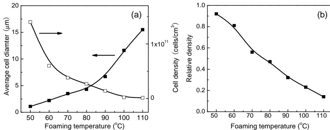
Fig. 5.2 (a) Effect of foaming temperature on cell morphology in terms of average cell size and cell density; (b) relative densities of PS foams as a function of foaming temperature.
