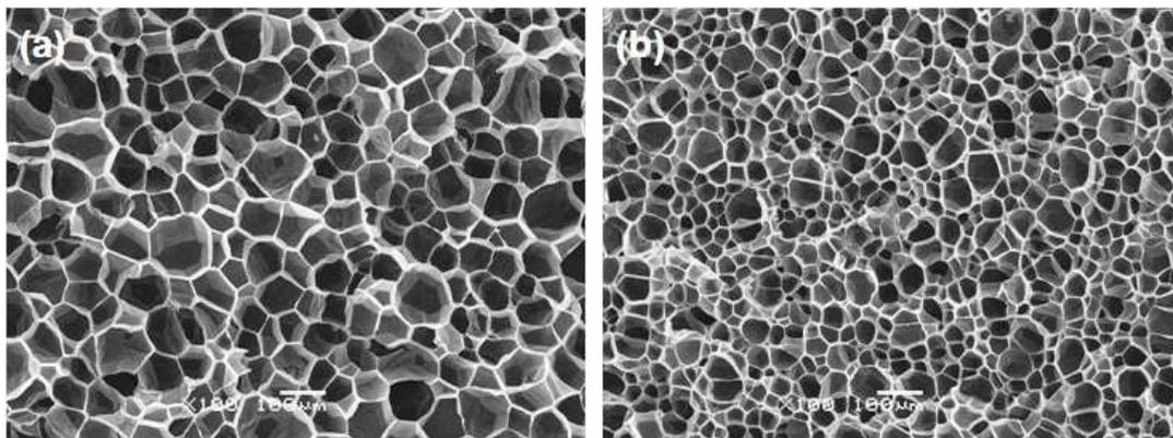
Fig. 4.13 SEM photographs of the skin and core layers foamed at 146 °C and a CO<sub>2</sub> pressure of 15MPa. (a) skin foam; and (b) core foam.
