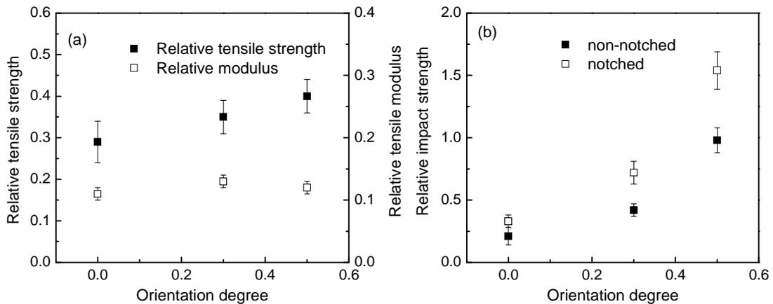
Fig. 5.14 Comparison of the mechanical properties of the c-oriented foams with different orientation degrees. The relative densities of the samples are all about  $0.3 \pm 0.02$ .
