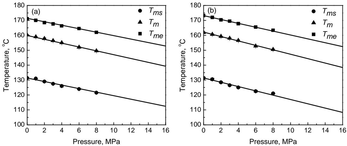
Fig. 4.7 Evolution of the starting melting temperature ( $T_{ms}$ ), melting temperature ( $T_m$ ) and ending melting temperature ( $T_{me}$ ) of the injection-molded iPP as a function of  $CO_2$  pressure. (a) skin layer,  $T_{ms}=131.8-1.33P$  (MPa);  $T_m=160.2-1.34P$ ;  $T_{me}=171.1-1.15P$ , and (b) core layer,  $T_{ms}=131.4-1.42P$ ;  $T_m=161.9-1.44P$ ;  $T_{me}=173.2-1.27P$ .
