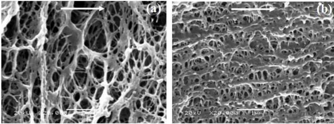
Fig. 3.8 SEM photographs of iPP samples in the shear zone foamed at 145 °C and a CO<sub>2</sub> saturation pressure of 15 MPa. (a): PP2; (b): PP6. White bars in (a) and (b) are 1 μm. The arrows indicate the flow direction.
