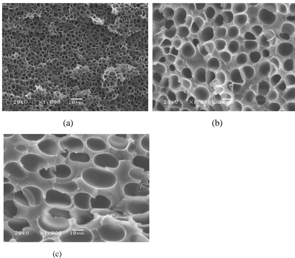
Fig. 5.8 SEM images of cell morphologies of PS foamed in the similar relative density of  $0.56 \pm 0.04$  with various average cell size: (a) 3.5  $\mu\text{m}$ , (b) 9.2  $\mu\text{m}$ , and (c) 15.8  $\mu\text{m}$ . The white bar is 10  $\mu\text{m}$ .
