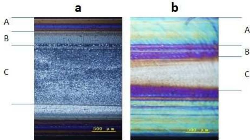
Fig. 3.3 Polarized optical micrographs of the cross-sections of the injection molded iPP samples at lower magnification: (a) PP1; (b) PP2. Distinct layers are: A: skin layer; B: intermediate layer and C: core layer.
