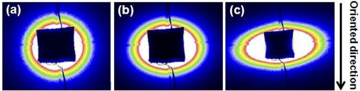
Fig. 5.17 2D SAXS images of PS foams with various c-axis orientation degree: (a) Orientation degree is 0; (b) orientation degree is 0.3; and (c) orientation degree is 0.5.
