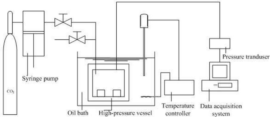
Fig. 2.1 Schematic of the CO<sub>2</sub> treatment apparatus.
