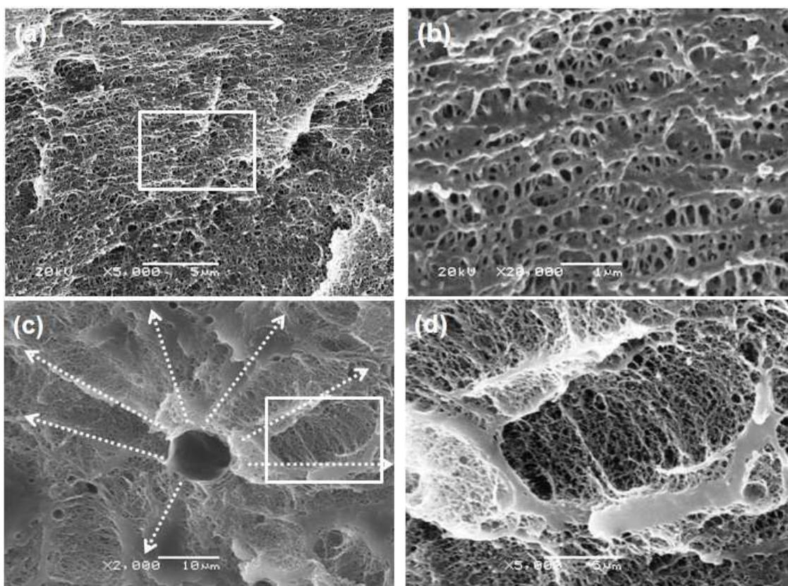
Fig. 4.10 SEM photographs of the skin and core layers foamed at 140 °C and a CO<sub>2</sub> saturation pressure of 15 MPa. (a) skin foam (the white arrow indicates the flow direction); (b) magnification of the white rectangle in part (a) (the white bar is 1 μm); (c) core foam; and (d) magnification of the white rectangle in part (c) (The white bar is 5μm).
