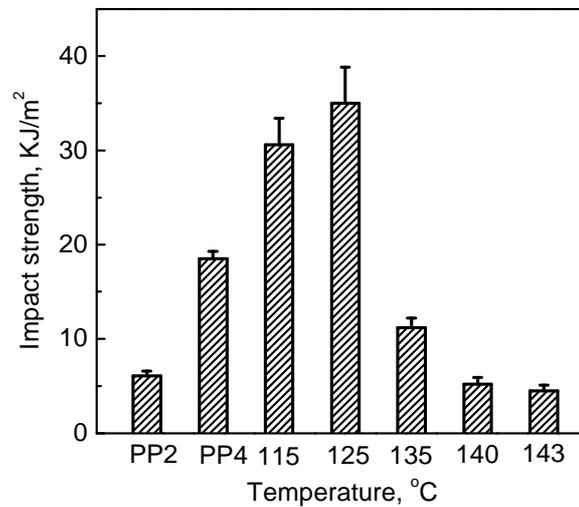
Fig. 4.14 Comparison of the impact strength of PP2 and PP4 with those of PP2 foamed under CO<sub>2</sub> pressure of 15MPa and various temperatures.
