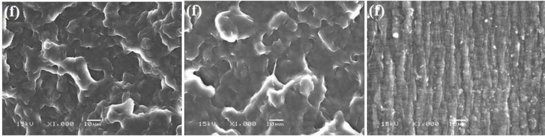
Fig.3.10 SEM images of the impact-fractured surface of PP1-PP6 at higher magnification. The images were obtained from the different zones as shown in Figure 10. (a) PP1, (b) PP2, (c) PP3, (d) PP4, (e) PP5 and (f) PP6.
