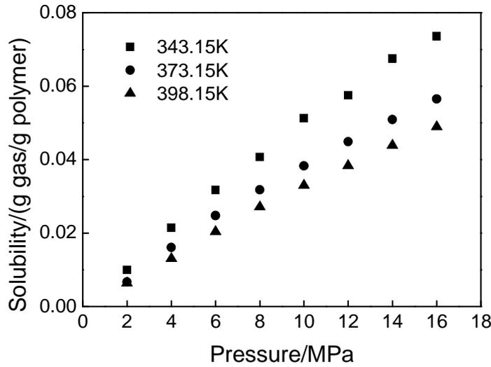
Fig. 3.16 Solubility of CO<sub>2</sub> in solid-state PP at various temperatures and pressures.
