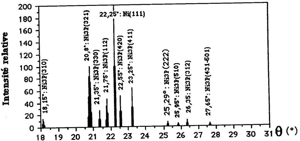
Figure 2F24(c): Diagramme R.X.(CuK $\alpha$ ) - Ech.13,5%AtP (Tr=350°C)
