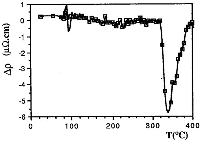
Figure 2F54:  $\Delta\rho$  de l'échantillon 15,5% AtP
