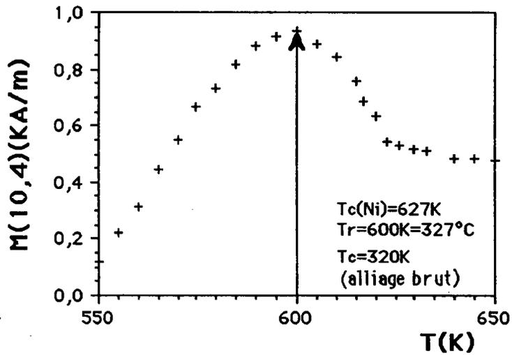
Figure 2F38(c): Transition de phase structurale, Ech.14,5% AtP
