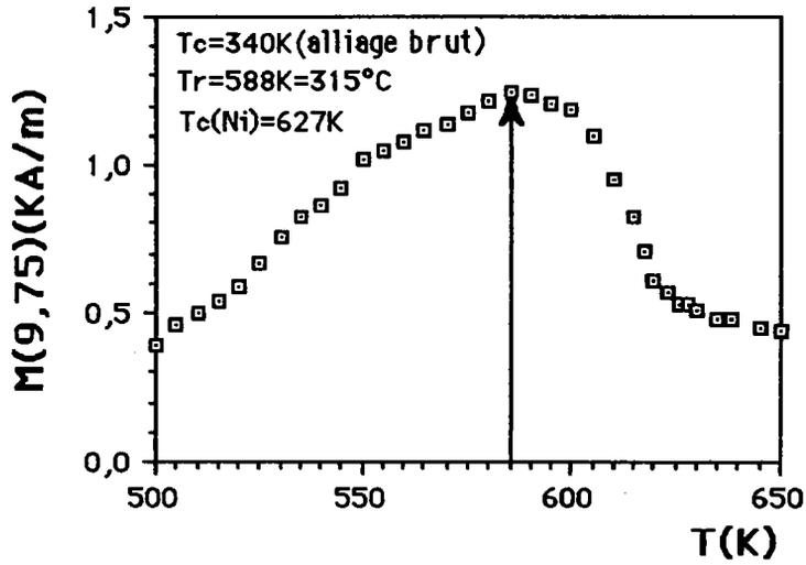
Figure 2F38(b): Transition de phase structurale, Ech.10,4% AtP
