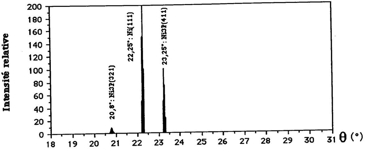
Figure 2F24(b): Diagramme R.X.(CuK $\alpha$ ) - Ech.10,5%AtP (Tr=350°C)
