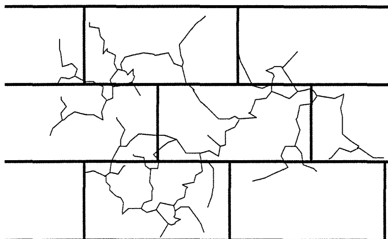
Figure 2-1. Microfissuration superficielle due aux variations de température
