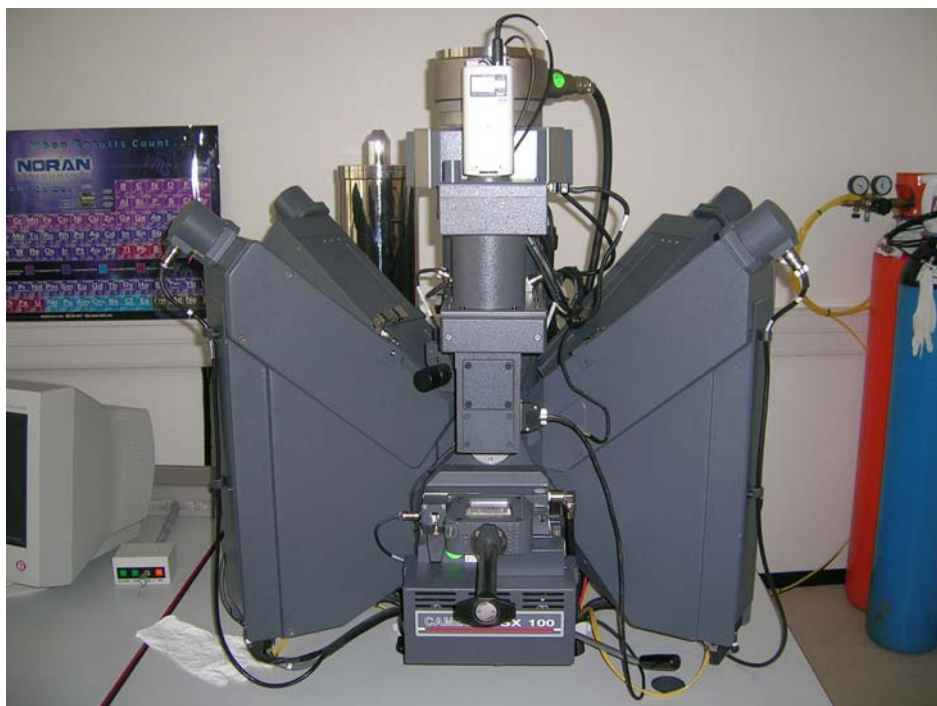
Figure 9 : microsonde de Castaing SX100 CAMECA
