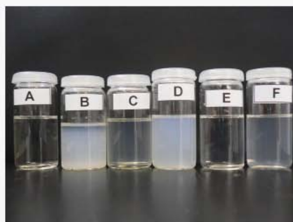
Fig. 1. Picture showing the macroscopic solubility in ethyl acetate of different nano- and microparticles prepared with different polymers: (A) ethyl acetate, (B) blank PCL nanoparticles, (C) EC/Eudragit® RS microparticles, (D) composite EC/Eudragit® RS microparticles, (E) simple Eudragit® RS microparticles, (F) simple EC microparticles.
