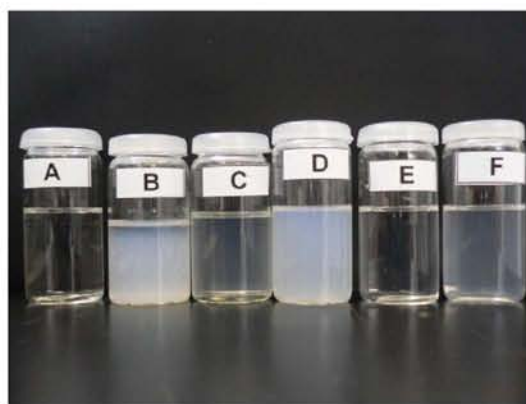
Fig. 1. Picture showing the macroscopic solubility in ethyl acetate of different nano- and microparticles prepared with different polymers: (A) ethyl acetate, (B) blank PCL nanoparticles, (C) EC/Eudragit® RS microparticles, (D) composite EC/Eudragit® RS microparticles, (E) simple Eudragit® RS microparticles, (F) simple EC microparticles.
