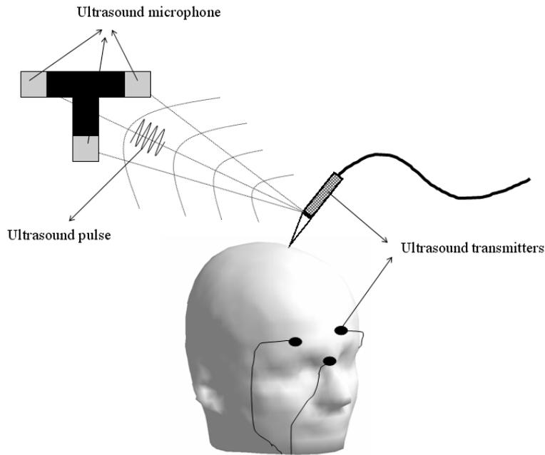
Fig. 5: Principle of Elpos system (Zebris, Tuebingen, Germany)
