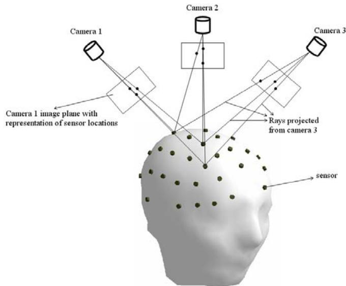
Fig. 7: Method for determination of 3D sensor position
