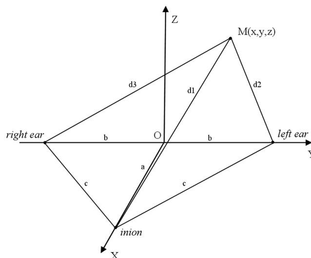
Fig. 1: Manual determination of the electrode position (M).
