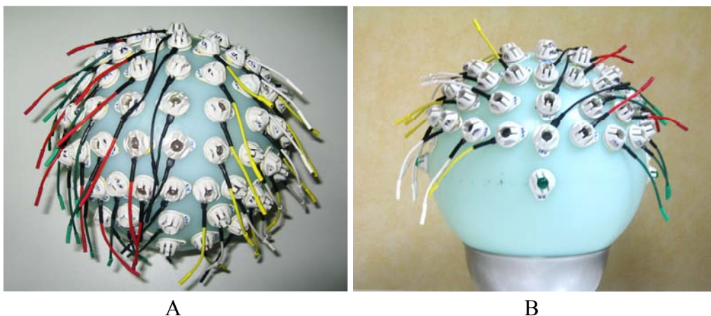
Fig. 5: Top (A) and front (B) views of 64 sensors taped on the MRI head phantom.
