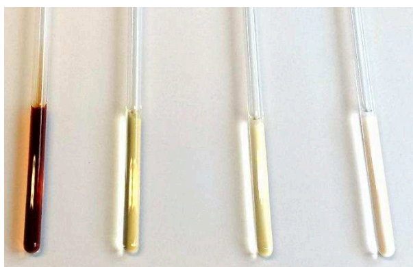
Figure III-35. Vanillin, trihydroxyacetophenone, cinnamaldehyde, and butyrophenone (from left to right) solutions after addition of \text{NH}_4\text{OH} and heating for 1 hour at 70 °C.
