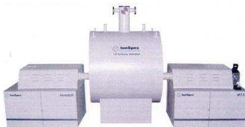
Figure II-24. Ion Spec FT-ICR mass spectrometer equipped with two external sources. LDI (on the left) and ESI (on the right).
