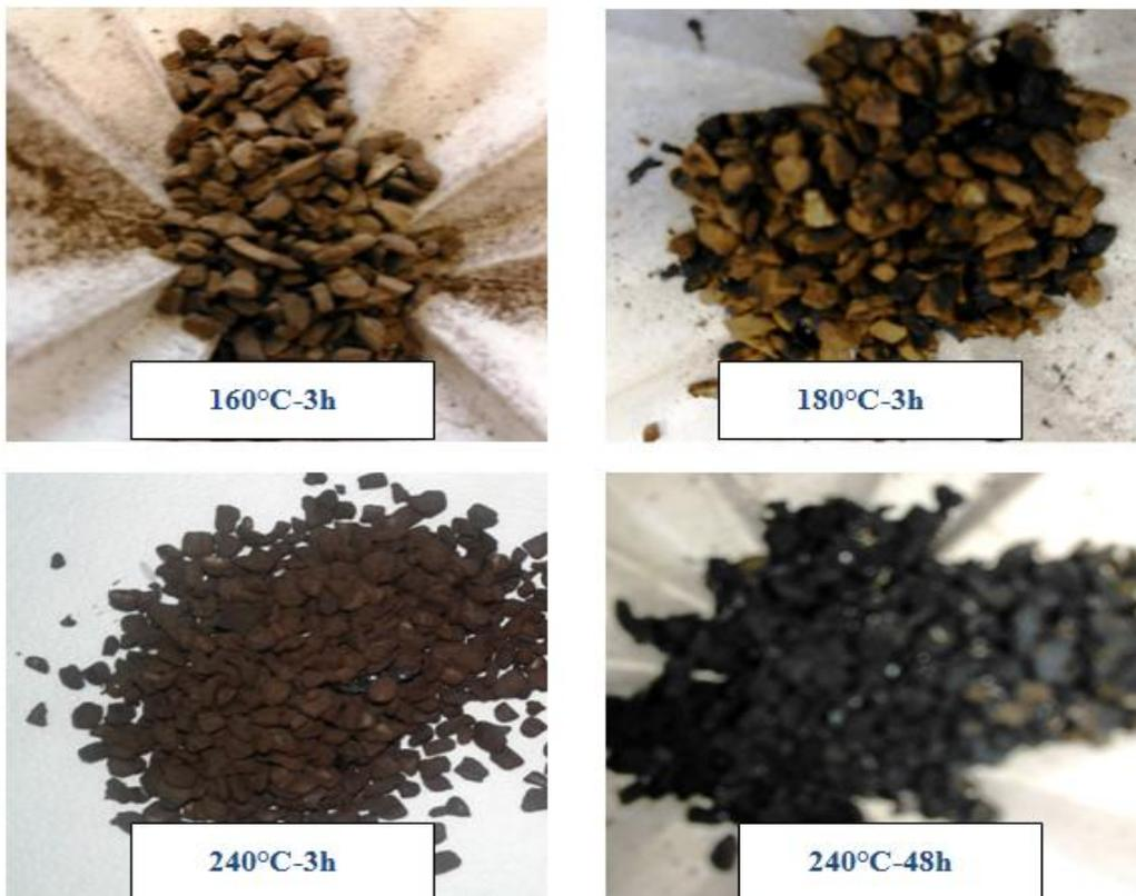
**Figure 17:** Hydrochar prepared at different temperature and time
