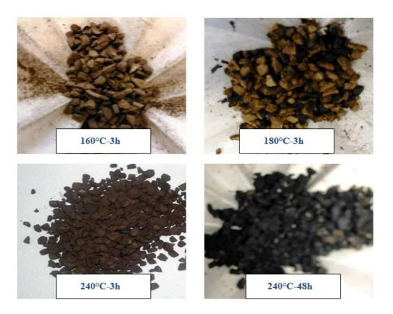
Figure 17: Hydrochar prepared at different temperature and time
