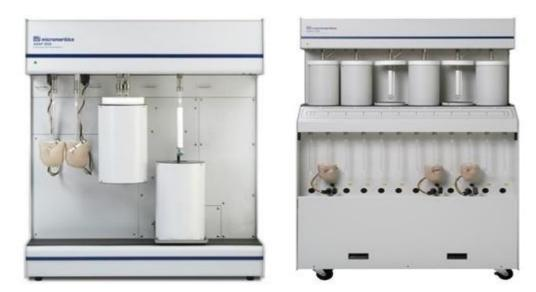
Figure 49: A photograph of ASAP 2020 (a) and ASAP 2420 (b) automatic equipment
