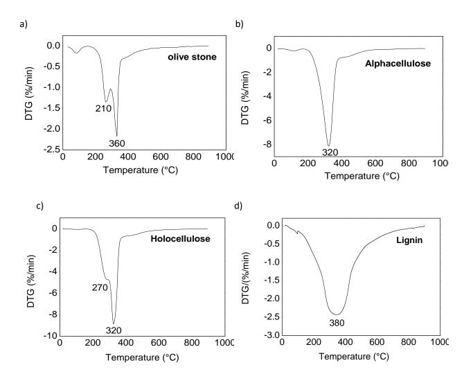
Figure 16: DTG curves of: a) olive stone, and of its three polymers: b) alpha-cellulose, c) holocellulose, and d) lignin
