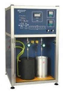
Figure 79: HPVA II - High Pressure apparatus Analyzer
