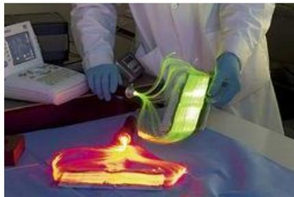
**Fig. 24:** Example on tissue-based light emitting fabric [87].
