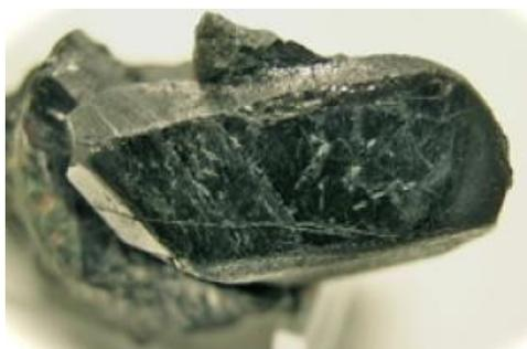
**Fig. 1:** Ilmenite ore. Picture obtained from virtual museum of the University of Huelva [1].
