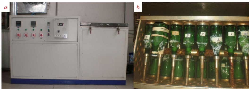
Figure 5-1. A shake-bottle polymerization device for PDIB elastomers. (a) Frontal view and (b) internal view.
