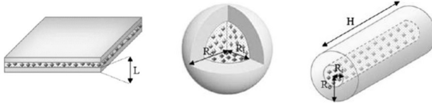
Fig. 1.14 Representations of reservoir devices (drug depot surrounded by a release rate controlling barrier membrane) at different geometries (slab, sphere, cylinder). Taken from [9]. Note that equations kinetics 1.6 and 1.7 are irrespective of the device geometry.
