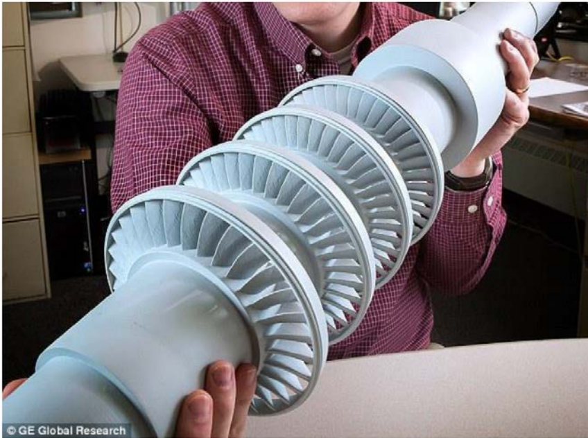
Figure 7: Scale of compressor for SC-CO 2 10 MWe test loop, photo extracted from GE company
