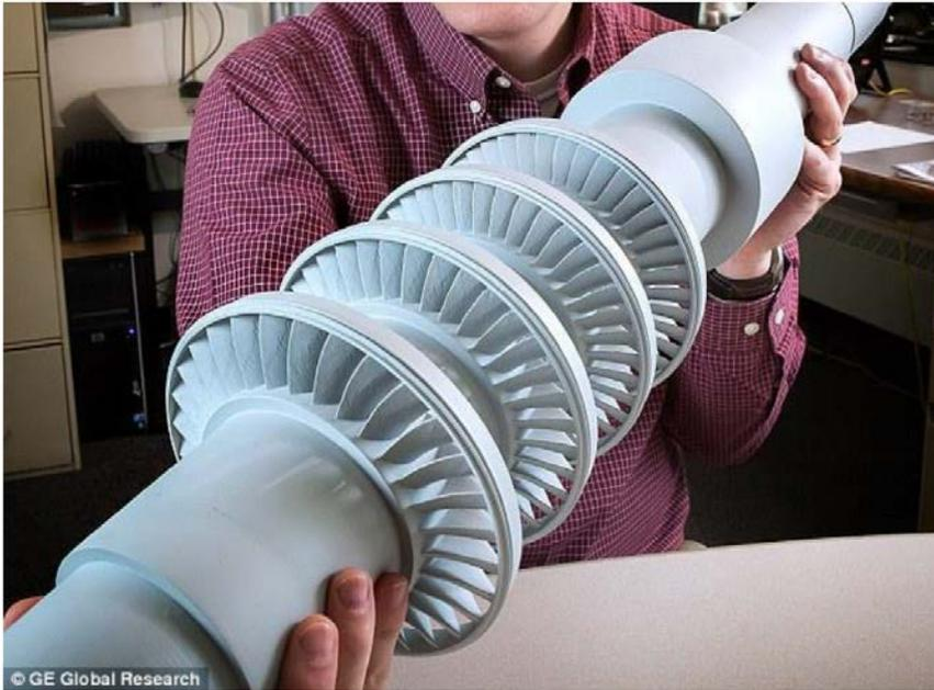
Figure 7: Scale of compressor for SC-CO<sub>2</sub> 10 MWe test loop, photo extracted from GE company
