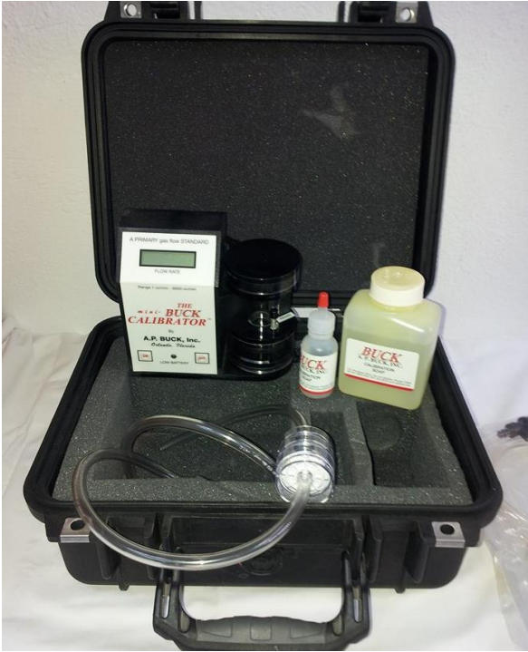
Figure 2.1: Equipment and materials for TME indoor air monitoring; a: Cassettes and quartz filters, b: sampling pump, c: calibrator
