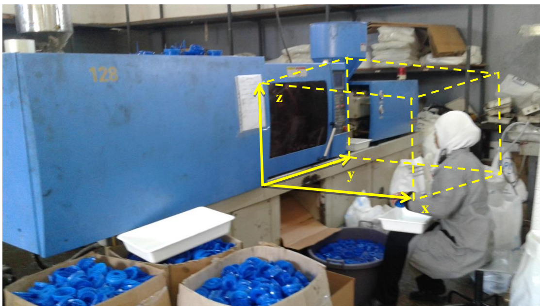
Figure 1.27: NF dimensions of P15 (plastic injection): x = 1.15 m, y = 1 m, z = 0.85 m
