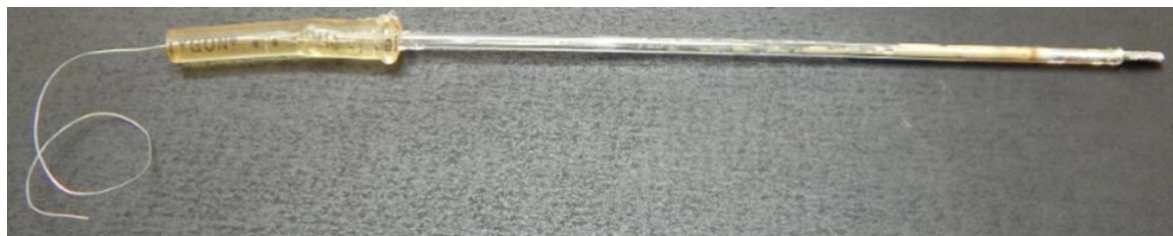
Figure 2.6: Platinum mesh based counter electrode
