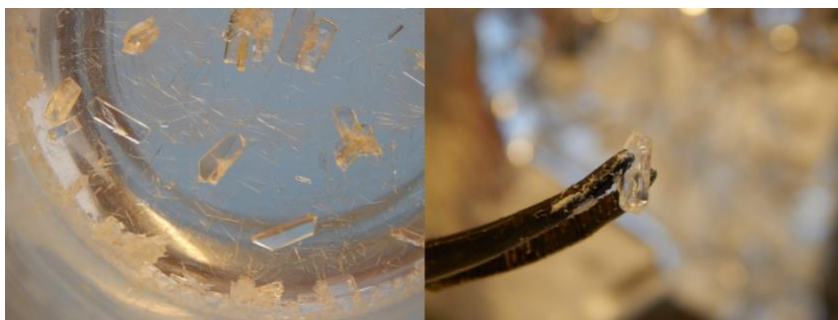
Figure 2.2: BTPPA + TPBCl - crystals after acetone evaporation
